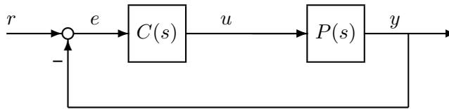
and let  $L(s) := P(s)C(s)$  denote the loop transfer function for the feedback system shown below. Consider two pairs of plants and controllers:
