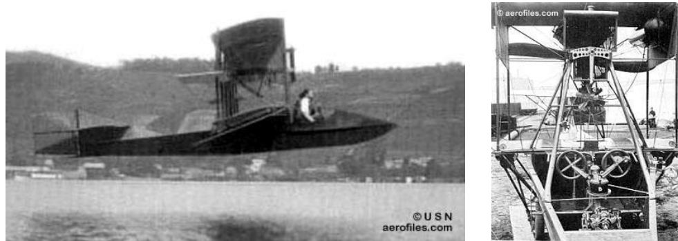
Figure 1.9: The Curtiss-Sperry E in 1912 (left) and a closeup of the Sperry Autopilot (right).
