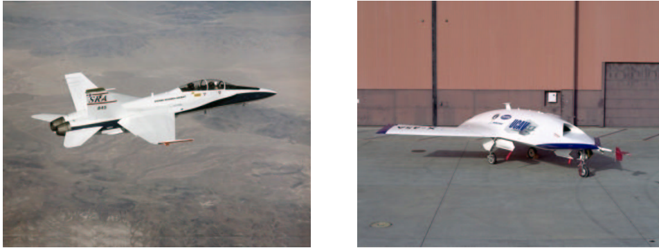
Figure 1.4: The F-18 aircraft, one of the first production military fighters to use “fly-by-wire” technology, and the X-45 (UCAV) unmanned aerial vehicle. Photographs courtesy of NASA Dryden Flight Research Center.
