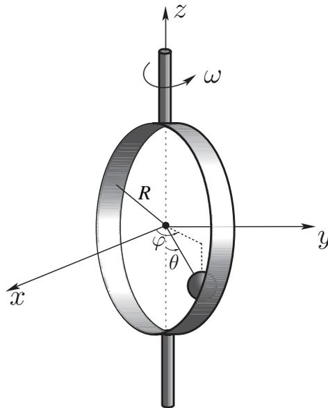
FIGURE 1.6.1. A particle moving in a rotating hoop.
