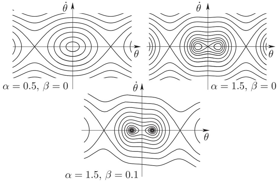
FIGURE 1.6.5. Phase portraits for the ball in the hoop. No damping, but increasing rotation rate as  $\alpha$  increases from  $\alpha = .05$  to  $\alpha = 1.5$  and  $\beta = 0$  and adding a bit of damping when  $\beta = 0.1$ .
