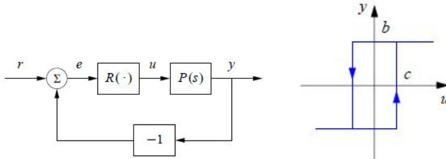
The block  $R$  is a relay with hysteresis whose input/output response is shown on the right and the process transfer function is  $P(s) = e^{-s\tau}/s$ . Use describing function analysis to determine frequency and amplitude of possible limit cycles. Simulate the system and compare with the results of the describing function analysis.
