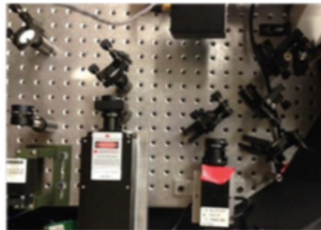
Dichroics and mirror assembly on the optical breadboard as per in the schematic
