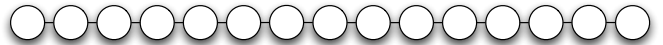
Fig. 3. The multi-agent system \mathcal{G} = (\mathcal{V}, \mathcal{E}) is communicating through a line topology. This topology has the maximal round-trip time among all networks with N agents.
