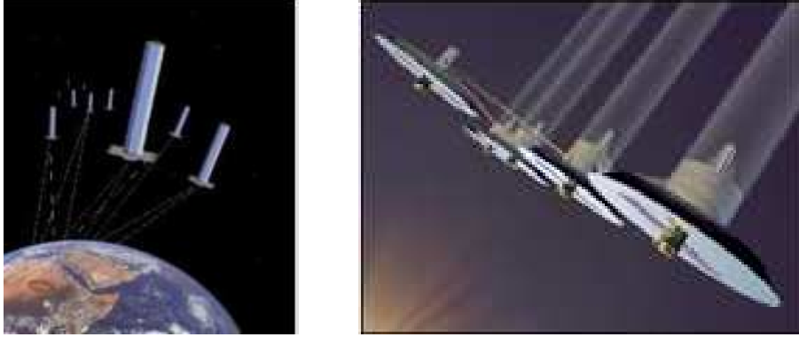
Figure 3: Distributed aperture observing systems: (a) the proposed TechSat 21 concept would use a collection of microsatellites to form the equivalent of a larger aperture imaging system; (b) the terrestrial planet finder uses formation flying to enable optimal interferometry for detecting planets.
