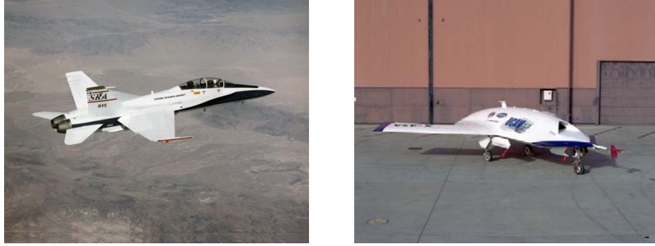
Figure 4: The F-18 aircraft, one of the first production military fighters to use “fly-by-wire” technology, and the X-45 (UCAV) unmanned aerial vehicle. Photographs courtesy of NASA Dryden Flight Research Center.
