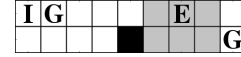
Fig. 11. Gridworld hallways. “I” is the robot initial position, each location marked with “G” must be visited infinitely often (like surveillance), and the shaded cell contains an obstacle that can move freely within it. The original maps, used for synthesizing nominal controllers, do not include the black walls.
