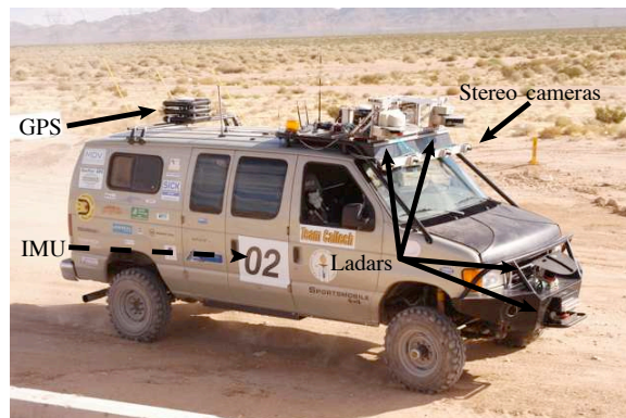
Fig. 1. Alice: Team Caltech's 2005 DGC entry. LADARs and cameras sense the terrain. The GPS and IMU units provide the vehicle state.
