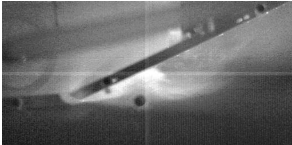
Figure 9: Top View of Diffuser with No Downstream Boundary Condition at Optimal Forcing.
