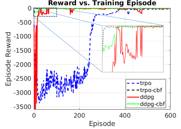
Figure 3: Accumulated reward from inverted pendulum problem using TRPO, DDPG, TRPO-CBF, and DDPG-CBF.
