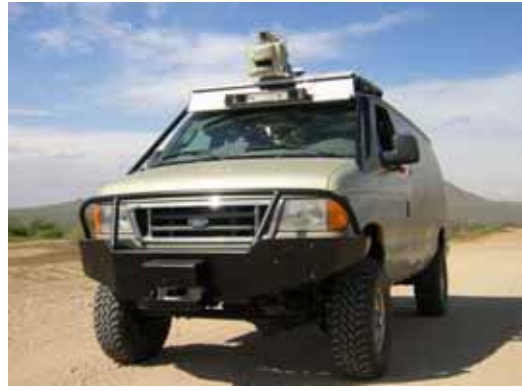
Fig. 5. Our test platform is a 2005 Ford E-350 Econoline van modified by Sportsmobile of Fresno, California. A roof-mounted LADAR and INS provide the raw data used for navigation of desert roads.
