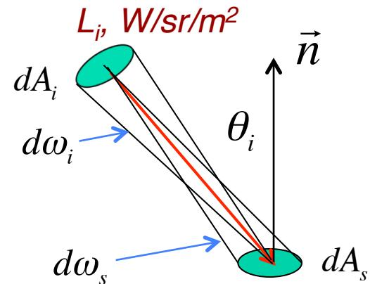
$$d\omega_s = \frac{dA_s \cos \theta_i}{r^2}, \quad d\omega_i = \frac{dA_i}{r^2}$$
