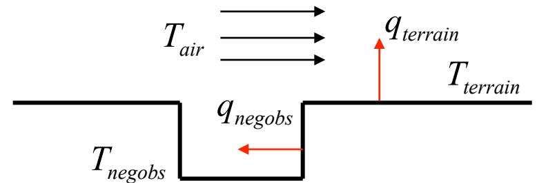
$$q_{terrain} = h(T_{terrain} - T_{air})$$
