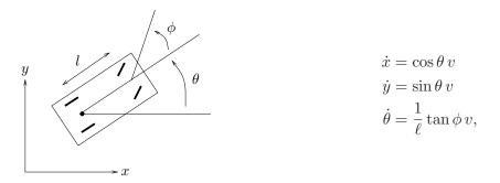
We assume that the vehicle is disturbance free, but that we have noisy measurements from the GPS receiver and IMU and an initial condition error.
