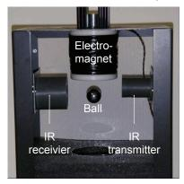
Process: actuation, sensing, dynamics
