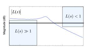
Transition between large gain and small gain complicated by stability (phase margin)
