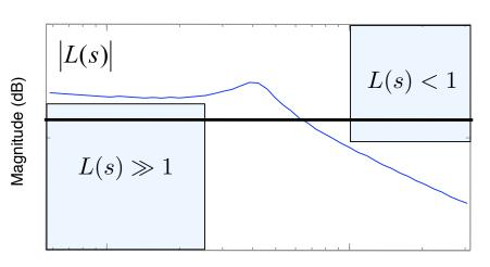
Transition between large gain and small gain complicated by stability (phase margin)
