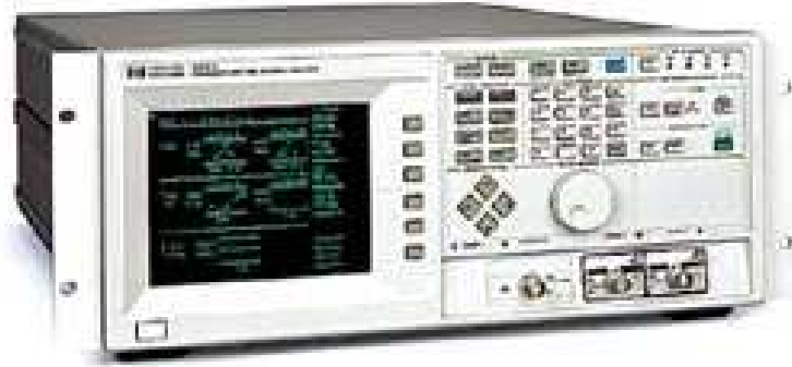
Figure 6.5: The Hewlett Packard signal analyzer can be used to determine frequency response experimentally.
