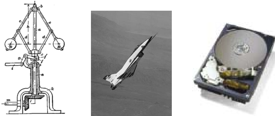
Figure 1: Applications of Control: (a) the Watt governor, (b) flight control and (c) disk drives.
