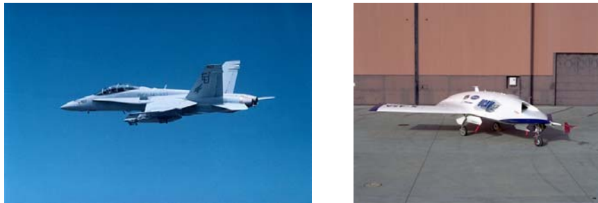
Figure 3.1. The F/A-18 aircraft, one of the first production military fighters to use “fly-by-wire” technology, and the X-45 (UCAV) unmanned aerial vehicle. (Figures courtesy NASA Dryden.)
