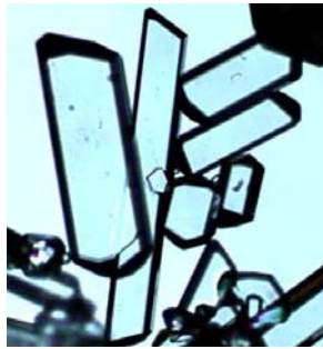
Figure 3.10. Microscope image of paracetamol crystals (paracetamol is the active ingredient in Tylenol), which shows the variability in crystal shape that can occur at a single time instance in a pharmaceutical crystallizer.
