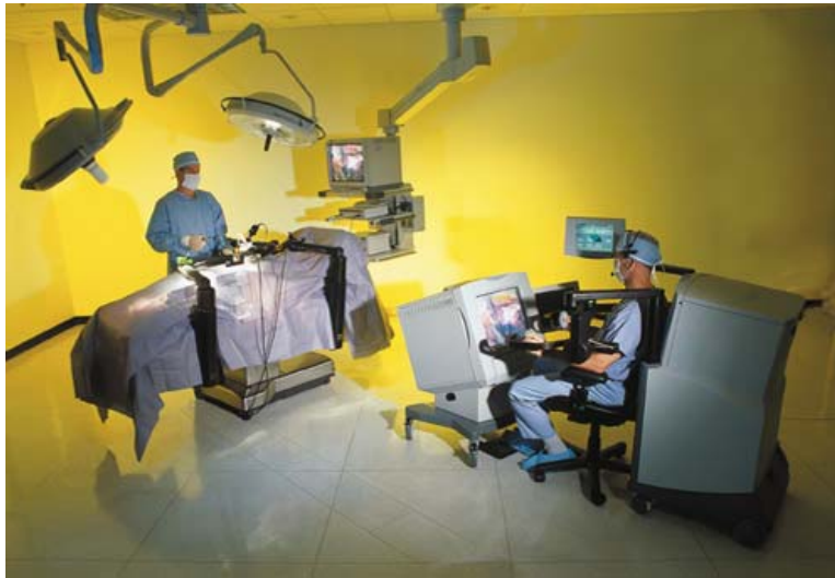
Figure 3.6. The ZEUS (tm) Robotic Surgical System, developed by Computer Motion Inc., is capable of performing minimally invasive microsurgery procedures from a remote location. (Photograph courtesy of Computer Motion Inc.)
