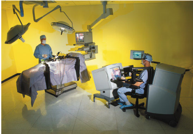
Figure 3.8. The ZEUS (tm) Robotic Surgical System, developed by Computer Motion Inc., is capable of performing minimally invasive microsurgery procedures from a remote location. Photograph courtesy of Computer Motion Inc.
