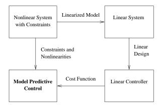
Figure 3.1: Optimization-based control approach.
