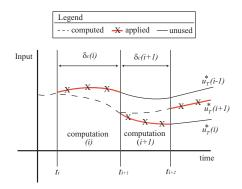
Figure 3.6: Receding horizon input trajectories
