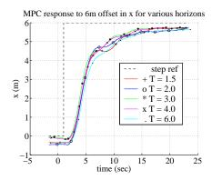
Figure 3.7: Receding horizon control: (a) moving one second average of computation time for MPC implementation with varying horizon time, (b) response of MPC controllers to 6 meter offset in x for different horizon lengths.
