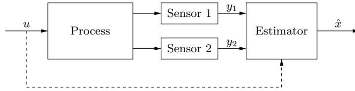
**Figure 7.1:** Sensor fusion. Multiple sensors report on data from a single process. The estimator fuses this information from the sensors to obtain an estimate of the state of the system. Depending on the use case, the input (dashed line) may not be available to the estimator.
