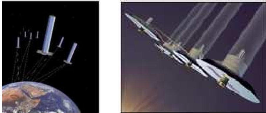
Figure 10.3: Distributed aperture observing systems: (a) the proposed TechSat 21 concept would use a collection of microsatellites to form the equivalent of a larger aperture imaging system; (b) the terrestrial planet finder uses formation flying to enable optimal interferometry for detecting planets.
