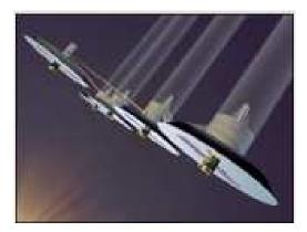
**Figure 10.3:** Distributed aperture observing systems: (a) the proposed TechSat 21 concept would use a collection of microsatellites to form the equivalent of a larger aperture imaging system; (b) the terrestrial planet finder uses formation flying to enable optimal interferometry for detecting planets.
