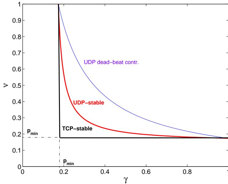
**Figure 6.10:** Region of convergence for UDP-like and TCP-like optimal control in the scalar case. The bounds are tight in the scalar case. The thin solid line corresponds to the boundary of the stability region for a dead-beat controller under UDP-like protocols as given by [?], which is much more restrictive than what can be achieved with optimal UDP controllers.
