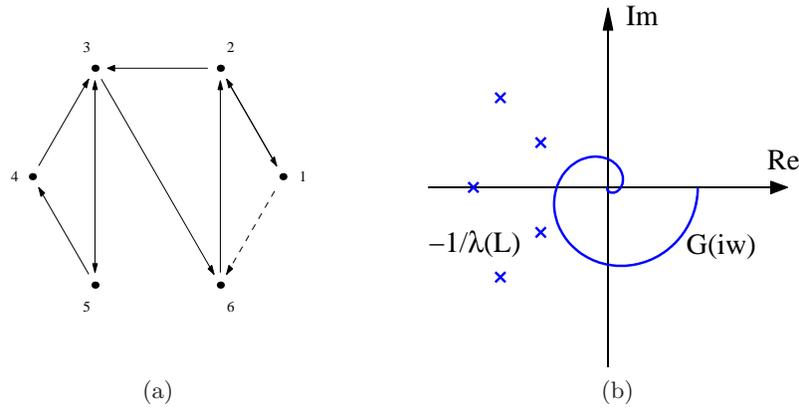
**Figure 9.1:** Interpretation of Theorem 1. The left figure shows the graph representation of the interconnected system and the right figure shows the corresponding Nyquist test. The addition of the dashed line to the graph moves the negative, inverse eigenvalues of  $\bar{L}$  from the positions marked by circles to those marked by crosses.
