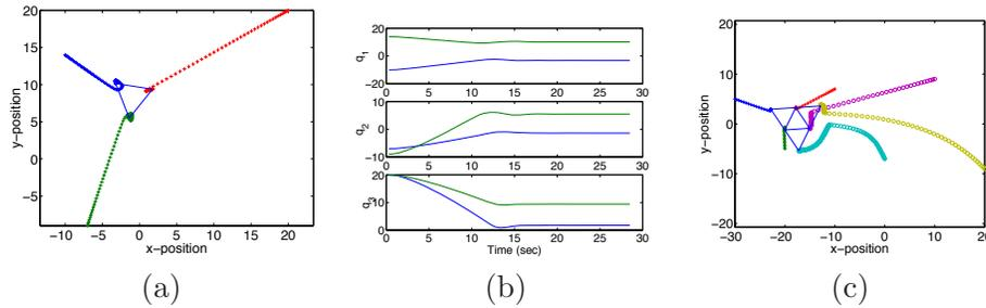
**Figure 10.7:** Formation stabilization using potential functions [OSM02]. (a) Stabilization of three vehicles in the plane. (b) Time traces for individual positions of the vehicles. (c) Stabilization of a six vehicle formation.
