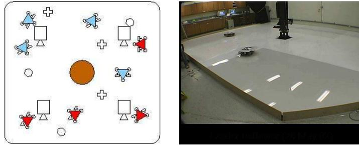
**Figure 1.3:** The Caltech Multi-Vehicle Wireless Testbed. The left figure shows the layout of the testbed area, including overhead cameras and fixed communication nodes (crosses and hexagons). The right picture is the current laboratory, with two vehicles shown.
