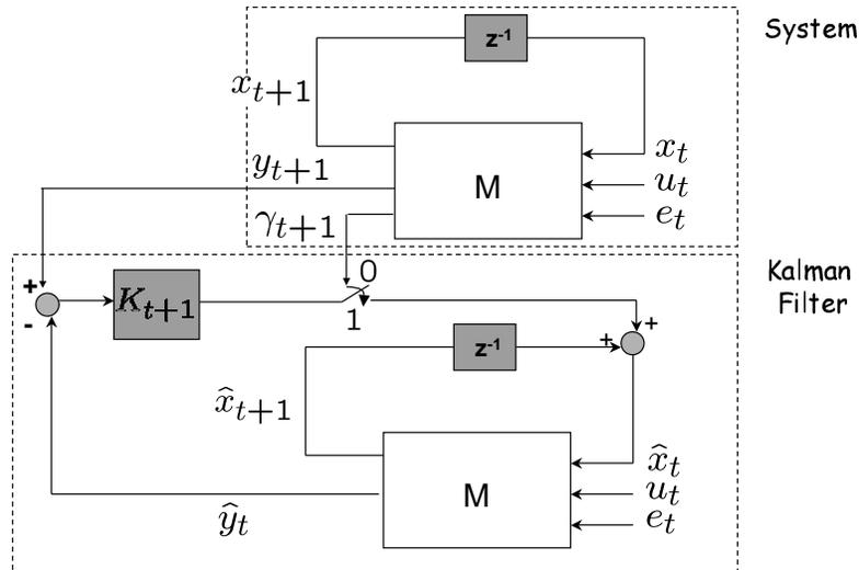
**Figure 6.1: Overview of the system.** The goal is to study the statistical convergence of the expected estimation error covariance of the discrete-time Kalman filter, where the observation, travelling over an unreliable communication channel, can be lost at each time step with probability  $1 - \bar{\gamma}$ .
