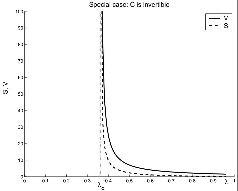
**Figure 6.2:** Example of transition to instability in the scalar case. The dashed line shows the asymptotic value of the lower bound ( $\bar{S}$ ), the solid line the asymptotic value of the upper bound ( $\bar{V}$ ), and the dash-dot line shows the asymptote ( $\gamma_c$ ).
