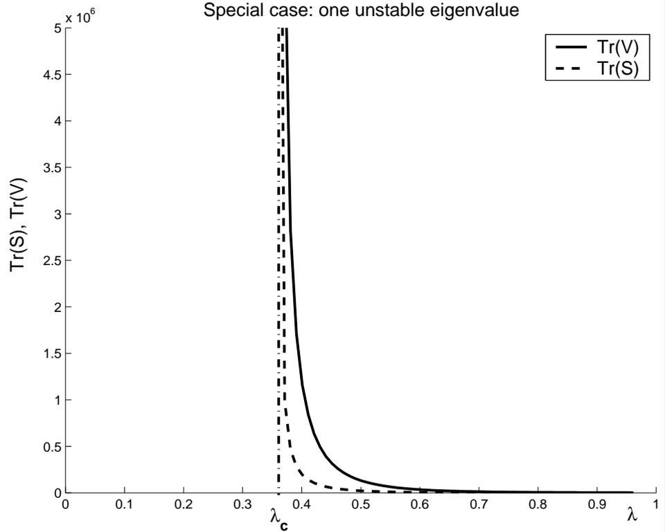
**Figure 6.3:** Example of transition to instability with a single unstable eigenvalue in the MIMO case. The dashed line shows the asymptotic value of the trace of lower bound ( $\bar{S}$ ), the solid line the asymptotic value of trace of the upper bound ( $\bar{V}$ ), and the dash-dot line shows the asymptote ( $\gamma_c$ ).
