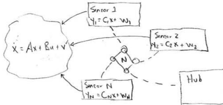
**Figure 8.1:** Schematic diagram of a distributed sensing system. The system on the left represents the system being observed. Multiple sensors take measurements and communication with each other across a communications network. A (optional) centralized hub collects information across the network.
