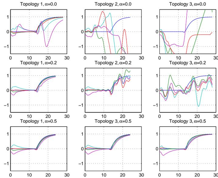
**Figure 10.8:** String stability results for a five vehicle formation [JM04]. Each column represents a different information topology, as shown in the diagram at the top of the column. The first row of plots corresponds to the use of purely local information, while the second two rows allow increasing amounts of global information.
