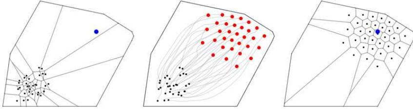
**Figure 10.14:** Coverage control applied to a polygonal region with Gaussian density function around the point in the upper right [?].
