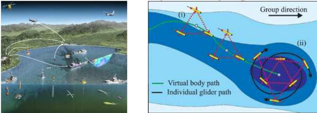
**Figure 10.2:** Autonomous ocean sampling network: (a) a depiction of the collection of vehicles that were part of the summer 2003 experiment; (b) an example of using a collection of gliders for sampling a region of interest.
