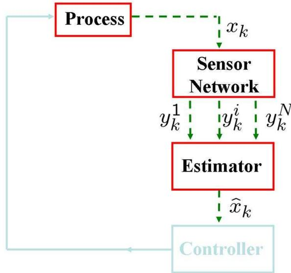
Figure 12.2: State Estimation Using a Wireless Sensor Network
