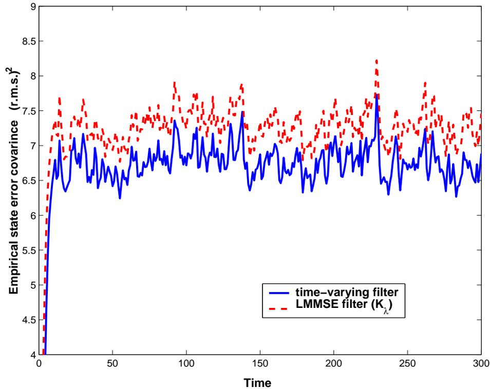
**Figure 6.7:** Empirical state error covariance of our time-varying filter and the linear minimum mean square error estimator (LMMSEE) [?] obtained by using the optimal static kalman gain  $K_{\bar{\gamma}}$ . The curves are obtained by averaging 10000 Monte Carlo simulations for  $t = 1, \dots, 300$ , with the values of the input noise  $(v_t, w_t)$  and the arrival sequence  $\gamma_t$  generated randomly. Both filters were compared under the same conditions.
