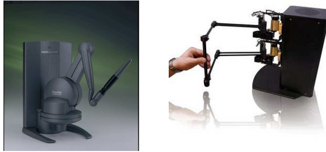
Figure 2.16: Haptic devices, the left figure shows the PHANTOM TM and the right a system is developed by Quanser.
