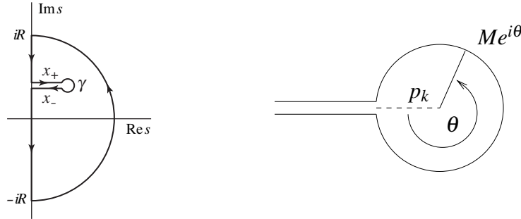
Figure 14.6: Contour used to prove Bode's theorem. For each right half-plane pole p_k of the loop transfer function L(s) , which is also a singularity of \log S(s) , we create a path from the imaginary axis that encircles the pole. To avoid clutter only one of the paths is shown.
