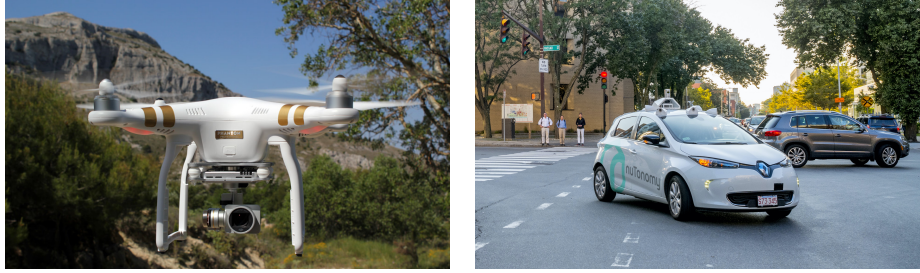
Figure 1.7: Autonomous vehicles. The figure on the left is a DJI Phantom 3 drone, which is able to maintain its position using GPS and inertial sensors. The figure on the right is an autonomous car that was developed by nuTonomy and is capable of driving on city streets by using sophisticated sensing and decision-making (control) software (photo courtesy Hyundai-Aptiv Autonomous Driving Joint Venture, LLC).
