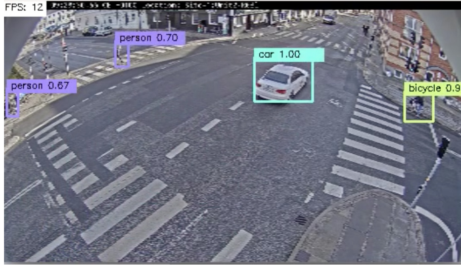
Figure 15.25: Illustration of feature detection based on deep learning. Objects are detected and classified as car, bicycle, or person, their position and spatial extent are also determined. The images typically have low-resolution to prevent identification of license plates and humans. The particular network which generated this figure has 13 layers and more than 25 million parameters [AJÅ + 17].
