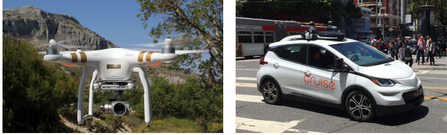
Figure 1.7: Autonomous vehicles. The figure on the left is a DJI Phantom 3 drone, which is able to maintain its position using GPS and inertial sensors. The figure on the right is an autonomous car that was developed by Cruise LLC and is capable of driving on city streets by using sophisticated sensing and decision-making (control) software.
