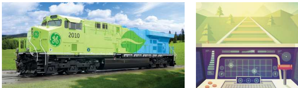
Figure 1.18: Freight locomotives carry massive loads of expensive diesel. GE's Trip Optimizer is a type of cruise control that combs through piles of data and synthesizes them for the driver in a way that allows him or her to steer the locomotive to maintain the most efficient speed at all times and reduce fuel burn.
