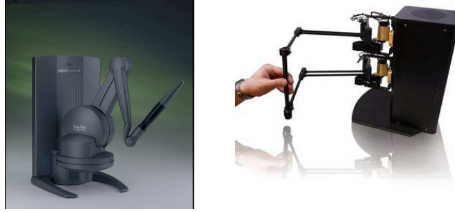
Figure 3.11: Haptic devices, the left figure shows the PHANTOM™ and the right a system is developed by Quanser.
