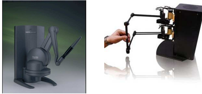
Figure 2.23: Haptic devices, the left figure shows the PHANTOM® and the right a system is developed by Quanser.
