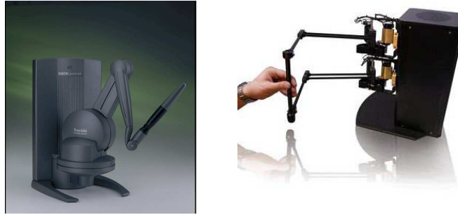
Figure 2.17: Haptic devices, the left figure shows the PHANTOM TM and the right a system is developed by Quanser.
