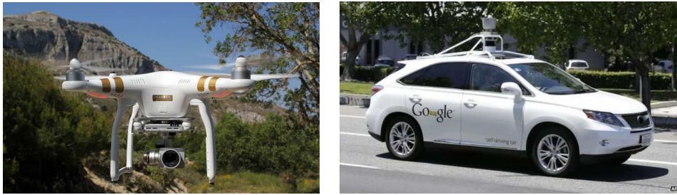
Figure 1.6: Autonomous vehicles. The figure on the left is a DJI Phantom 3 drone, which is able to maintain its position using GPS and inertial sensors. The figure on the right is an autonomous car that was developed by Google and is capable of driving on city streets by using sophisticated sensing and decision-making (control) software.
