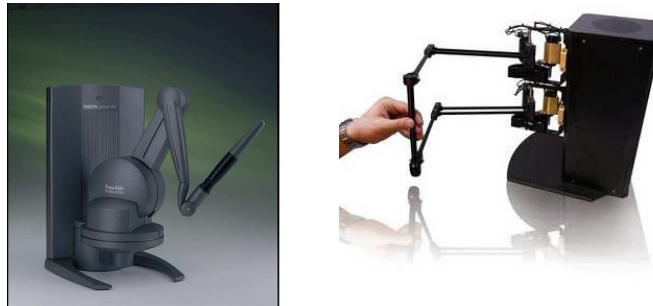
Figure 3.11: Haptic devices, the left figure shows the Phantom and the right a system from Quanser.
