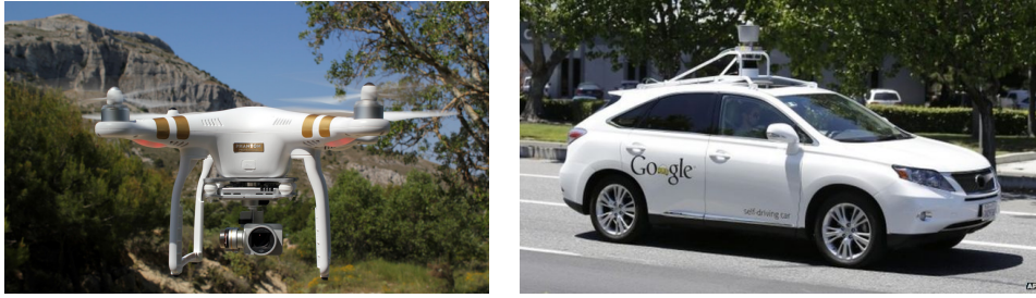
Figure 1.7: Autonomous vehicles. The figure on the left is a DJI Phantom 3 drone, which is able to maintain its position using GPS and inertial sensors. The figure on the right is an autonomous car that was developed by Google and is capable of driving on city streets by using sophisticated sensing and decision-making (control) software.
