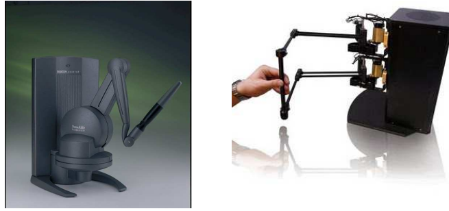
Figure 3.22: Haptic devices, the left figure shows the PHANTOM® and the right a system is developed by Quanser.
