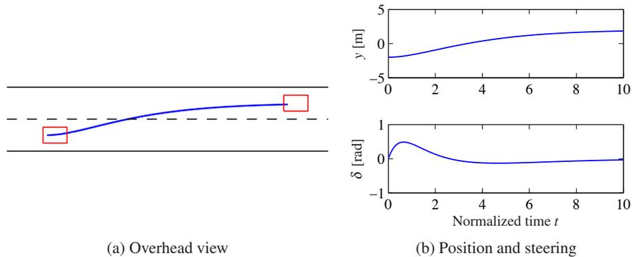
**Figure 12.4:** Feedforward control for vehicle steering. The plot on the left shows the trajectory generated by the controller for changing lanes. The plots on the right show the lateral deviation  $y$  (top) and the steering angle  $\delta$  (bottom) for a smooth lane change control using feedforward (based on the linearized model).
