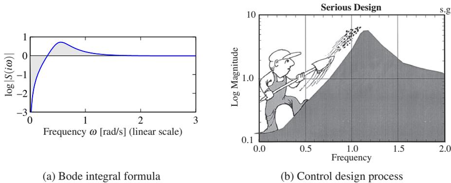
**Figure 12.16:** Interpretation of the *waterbed effect*. The function  $\log |S(i\omega)|$  is plotted versus  $\omega$  in linear scales in (a). According to Bode's integral formula (12.25), the area of  $\log |S(i\omega)|$  above zero must be equal to the area below zero. Gunter Stein's interpretation of design as a trade-off of sensitivities at different frequencies is shown in (b) (from [Ste03]).
