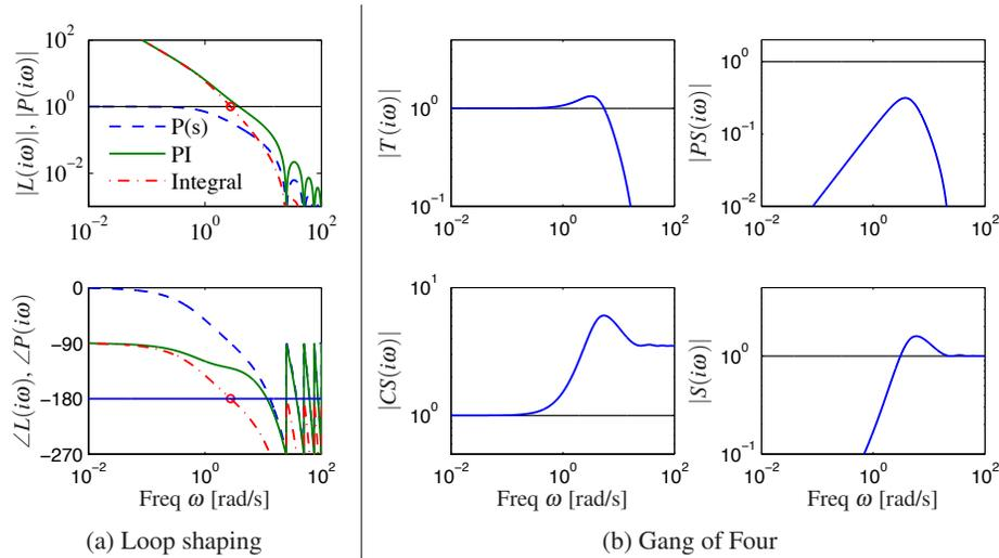
**Figure 12.10:** Loop-shaping design of a controller for an atomic force microscope in tapping mode. (a) Bode plots of the process (dashed), the loop transfer function for an integral controller with critical gain (dash-dotted) and a PI controller (solid) adjusted to give reasonable robustness. (b) Gain curves for the Gang of Four for the system.
