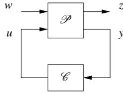
**Figure 12.2:** A more general representation of a feedback system. The process input  $u$  represents the control signal, which can be manipulated, and the process input  $w$  represents other signals that influence the process. The process output  $y$  is the vector of measured variables and  $z$  are other signals of interest.
