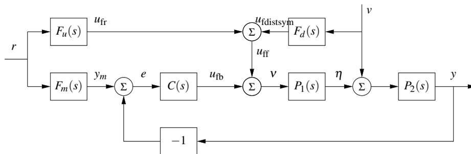
**Figure 12.3:** Block diagram of a system with feedforward compensation for improved response to reference signals and measured disturbances (2 DOF system). Three feedforward elements are present:  $F_m(s)$  sets the desired output value,  $F_u(s)$  generates the feedforward command  $u_{fr}$  and  $F_d(s)$  attempts to cancel disturbances.
