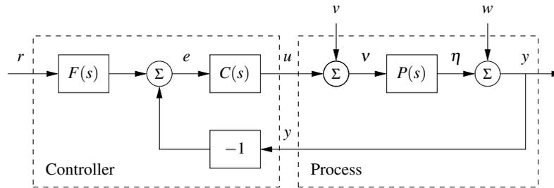
**Figure 12.1:** Block diagram of a basic feedback loop with two degrees of freedom. The controller has a feedback block  $C$  and a feedforward block  $F$ . The external signals are the reference signal  $r$ , the load disturbance  $v$  and the measurement noise  $w$ . The process output is  $\eta$ , and the control signal is  $u$ .
