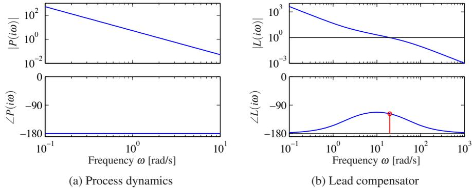
**Figure 12.12:** Control design for a vectored thrust aircraft using lead compensation. The Bode plot for the open loop process  $P$  is shown in (a) and for the loop transfer function  $L = PC$  using a lead compensator  $C$  in (b). Note the phase lead in the crossover region near  $\omega = 100$  rad/s.
