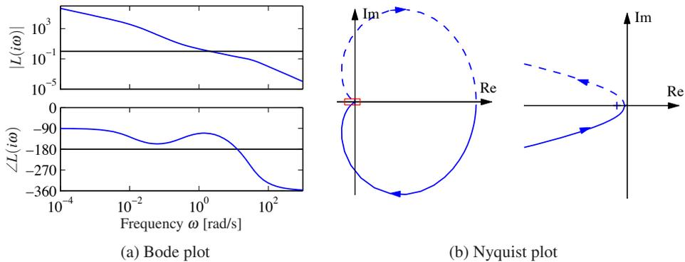
**Figure 12.21:** Inner/outer loop controller for a vectored thrust aircraft. Bode plot (a) and Nyquist plot (b) for the loop transfer function cut at  $\theta_d$ , for the complete system. The system has a phase margin of  $68^\circ$  and a gain margin of 6.2.
