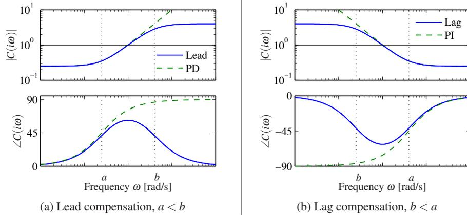
**Figure 12.9:** Frequency response for lead and lag compensators  $C(s) = k(s + a)/(s + b)$ . Lead compensation (a) occurs when  $a < b$  and provides phase lead between  $\omega = a$  and  $\omega = b$ . Lag compensation (b) corresponds to  $a > b$  and provides low-frequency gain. PI control is a special case of lag compensation and PD control is a special case of lead compensation. PI/PD frequency responses are shown by dashed curves.
