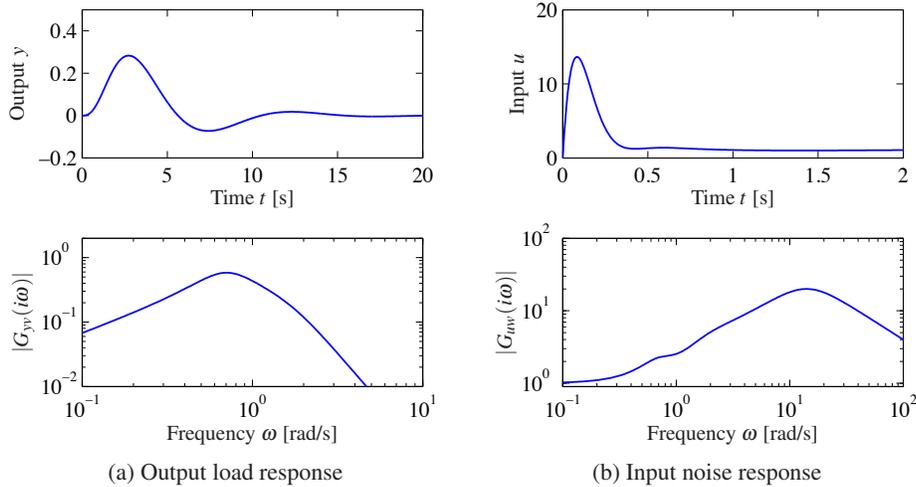
**Figure 12.7:** Closed loop disturbance responses. The time and frequency responses of process output  $y$  to load disturbance  $v$  are shown in (a) and the responses of control signal  $u$  to measurement noise  $w$  are shown in (b).
