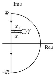
**Figure 12.18:** Contour used to prove Bode's theorem. For each right half-plane pole we create a path from the imaginary axis that encircles the pole as shown. To avoid clutter we have shown only one of the paths that enclose one right half-plane.
