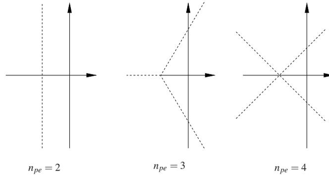
**Figure 12.13:** Asymptotes of root locus for systems with pole excess  $n_{pe} = 2, 3$  and  $4$ . There are  $n_{pe}$  asymptotes radiate from the point given by equation 12.15, and the angles between the asymptotes are  $2\pi/n_{pe}$ .
