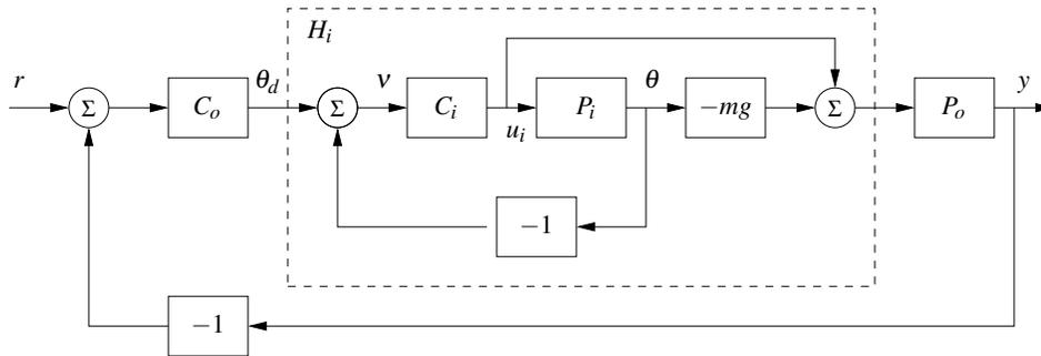
**Figure 12.19:** Inner/outer control design for a vectored thrust aircraft. The inner loop  $H_i$  controls the roll angle of the aircraft using the vectored thrust. The outer loop controller  $C_o$  commands the roll angle to regulate the lateral position. The process dynamics are decomposed into inner loop ( $P_i$ ) and outer loop ( $P_o$ ) dynamics, which combine to form the full dynamics for the aircraft.
