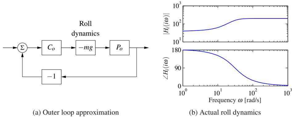
**Figure 12.20:** Outer loop control design for a vectored thrust aircraft. (a) The outer loop approximates the roll dynamics as a state gain  $-mg$ . (b) The Bode plot for the roll dynamics, indicating that this approximation is accurate up to approximately 10 rad/s.
