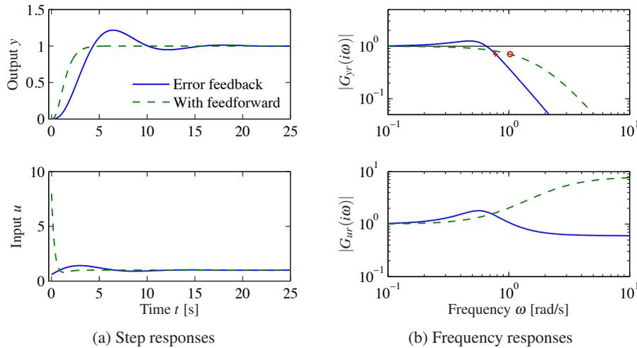
**Figure 12.5:** Reference signal responses. The responses in process output  $y$  and control signal  $u$  to a unit step in the reference signal  $r$  are shown in (a), and the gain curves of  $G_{yr}$  and  $G_{ur}$  are shown in (b). Results with PI control with error feedback are shown by solid lines, and the dashed lines show results for a controller with a feedforward compensator.
