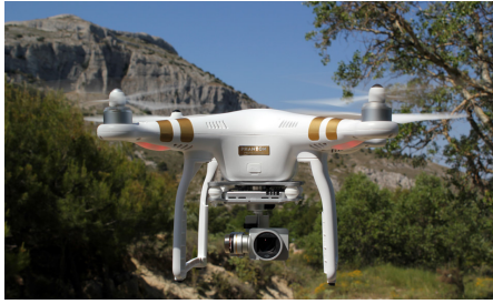
Figure 1.7: Autonomous vehicles. The figure on the left is a DJI Phantom 3 drone, which is able to maintain its position using GPS and inertial sensors. The figure on the right is an autonomous car that was developed by Google and is capable of driving on city streets by using sophisticated sensing and decision-making (control) software.
