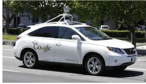
Figure 1.7: Autonomous vehicles. The figure on the left is a DJI Phantom 3 drone, which is able to maintain its position using GPS and inertial sensors. The figure on the right is an autonomous car that was developed by Google and is capable of driving on city streets by using sophisticated sensing and decision-making (control) software.
