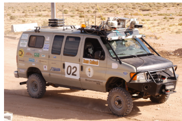
Figure 1.23: DARPA Grand Challenge. "Alice," Team Caltech's entry in the 2005 and 2007 competitions and its networked control architecture [CFG+06].
