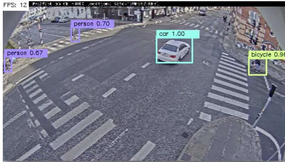
Figure 15.24: Illustration of feature detection based on deep learning. Objects are detected and classified as car, bicycle, or person, their position and spatial extent are also determined. The images typically have low-resolution to prevent identification of license plates and humans. The particular network which generated this figures has 13 layers and more than 25 million parameters [?].
