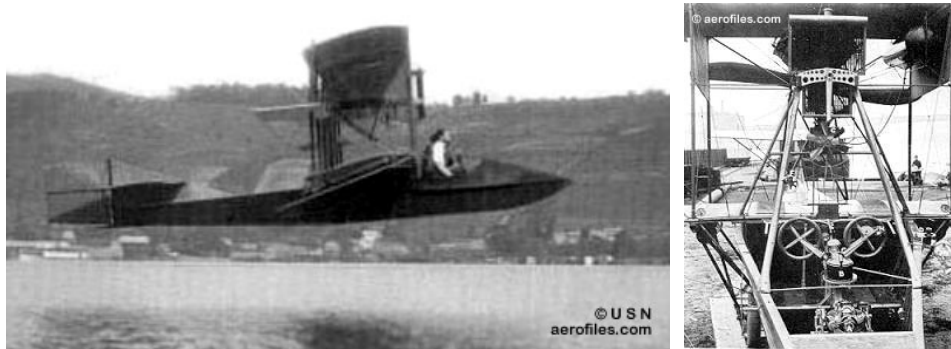
Figure 1.14: Aircraft autopilot system. The 1912 Curtiss (left) used an autopilot to stabilize the pitch of the aircraft. The Sperry Autopilot (right) contained a set of four gyros coupled to a set of air valves that controlled the wing surfaces. The Sperry Autopilot was able to correct for errors in roll, pitch and yaw [100].
