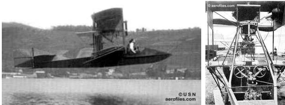
Figure 1.14: Aircraft autopilot system. The 1912 Curtiss (left) used an autopilot to stabilize the pitch of the aircraft. The Sperry Autopilot (right) contained a set of four gyros coupled to a set of air valves that controlled the wing surfaces. The Sperry Autopilot was able to correct for errors in roll, pitch and yaw [99].
