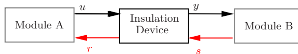
Figure 6.10: An insulation device is placed between an upstream module A and a downstream module B in order to protect these systems from retroactivity. An insulation device should have r \approx 0 and the dynamic response of y to u should be practically independent of s .
