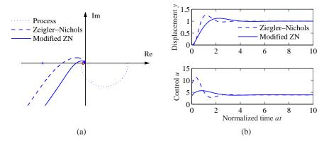
**Figure 10.8:** PI control of an AFM in tapping mode. Nyquist plots (a) and step responses (b) for PI control of the vertical motion of an atomic force microscope in tapping mode. The averaging parameter is n=20. Results with Ziegler–Nichols tuning are shown by dashed lines, and modified Ziegler–Nichols tuning is shown by solid lines. The Nyquist plot of the process transfer function is shown by dotted lines.
