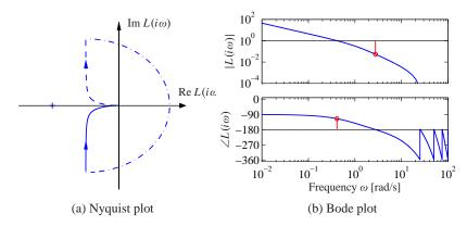
**Figure 10.5:** Integral control for AFM in tapping mode. An integral controller is designed based on the slope of the process transfer function at 0. The controller gives good robustness properties based on a very simple analysis.
