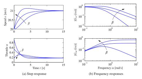
**Figure 10.12:** Time and frequency responses for PI cruise control with setpoint weighting. Step responses are shown in (a), and the gain curves of the frequency responses in (b). The controller gains are  $k_p = 0.74$  and  $k_i = 0.19$ . The setpoint weights are  $\beta = 0$ , 0.5 and 1, and  $\gamma = 0$ .
