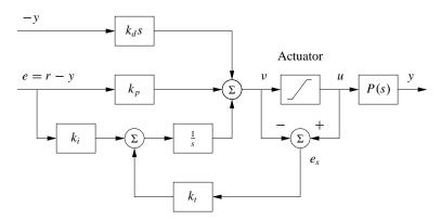
**Figure 10.11:** PID controller with a filtered derivative and anti-windup. The input to the integrator (1/s) consists of the error term plus a "reset" based on input saturation. If the actuator is not saturated, then  $e_s = u - v$ , otherwise  $e_s$  will decrease the integrator input to prevent windup.
