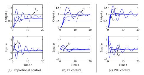
**Figure 10.2:** Responses to step changes in the reference value for a system with a proportional controller (a), PI controller (b) and PID controller (c). The process has the transfer function  $P(s) = 1/(s+1)^3$ , the proportional controller has parameters  $k_p = 1, 2$  and 5, the PI controller has parameters  $k_p = 1, k_i = 0, 0.2, 0.5$  and 1, and the PID controller has parameters  $k_p = 2.5$ ,  $k_i = 1.5$  and  $k_d = 0, 1, 2$  and 4.
