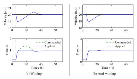
**Figure 10.10:** Simulation of PI cruise control with windup (a) and anti-windup (b). The figure shows the speed v and the throttle u for a car that encounters a slope that is so steep that the throttle saturates. The controller output is a dashed line. The controller parameters are  $k_p = 0.5$  and  $k_i = 0.1$ . The anti-windup compensator eliminates the overshoot by preventing the error for building up in the integral term of the controller.
