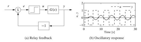
**Figure 10.9:** Block diagram of a process with relay feedback (a) and typical signals (b). The process output y is a solid line, and the relay output u is a dashed line. Notice that the signals u and y have opposite phases.
