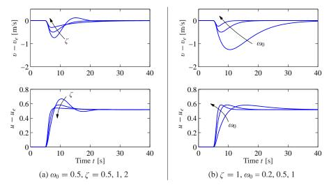
**Figure 10.6:** Cruise control using PI feedback. The step responses for the error and input illustrate the effect of parameters  $\zeta=1$  and  $\omega_0$  on the response of a car with cruise control. A change in road slope from  $0^\circ$  to  $4^\circ$  is applied between t=5 and 6 s. (a) Responses for  $\omega_0=0.5$  and  $\zeta=0.5$ , 1 and 2. Choosing  $\zeta=1$  gives no overshoot. (b) Responses for  $\zeta=1$  and  $\omega_0=0.2$ , 0.5 and 1.0.
