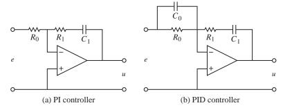
**Figure 10.13:** Schematic diagrams for PI and PID controllers using op amps. The circuit in (a) uses a capacitor in the feedback path to store the integral of the error. The circuit in (b) adds a filter on the input to provide derivative action.
