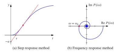
**Figure 10.7:** Ziegler–Nichols step and frequency response experiments. The unit step response in (a) is characterized by the parameters a and  $\tau$ . The frequency response method (b) characterizes process dynamics by the point where the Nyquist curve of the process transfer function first intersects the negative real axis and the frequency  $\omega_c$  where this occurs.
