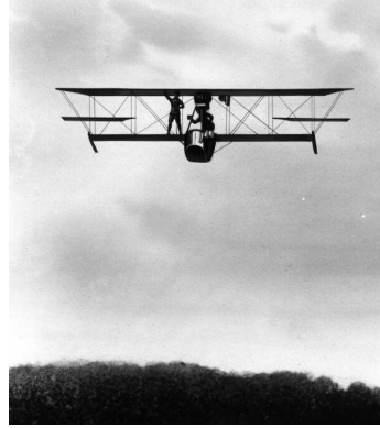
Figure 1.14: Aircraft autopilot system. The Sperry autopilot (left) contained a set of four gyros coupled to a set of air valves that controlled the wing surfaces. The 1912 Curtiss used an autopilot to stabilize the roll, pitch and yaw of the aircraft and was able to maintain level flight as a mechanic walked on the wing (right) [Hug93].
