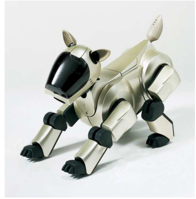
Figure 1.9: Robotic systems. (a) Spirit, one of the two Mars Exploratory Rovers that landed on Mars in January 2004. (b) The Sony AIBO Entertainment Robot, one of the first entertainment robots to be mass-marketed. Both robots make use of feedback between sensors, actuators and computation to function in unknown environments. (Photographs courtesy of Jet Propulsion Laboratory and Sony Electronics, Inc.)
