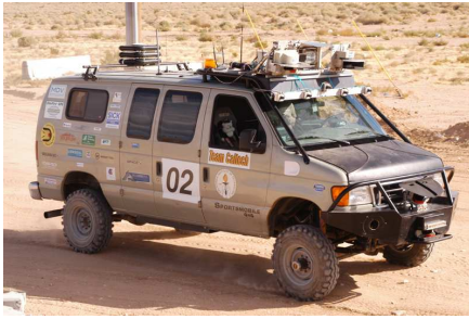
Figure 1.15: DARPA Grand Challenge. “Alice,” Team Caltech’s entry in the 2005 and 2007 competitions and its networked control architecture [CFG+06]. The feedback system fuses data from terrain sensors (cameras and laser range finders) to determine a digital elevation map. This map is used to compute the vehicle’s potential speed over the terrain, and an optimization-based path planner then commands a trajectory for the vehicle to follow. A supervisory control module performs higher-level tasks such as handling sensor and actuator failures.
