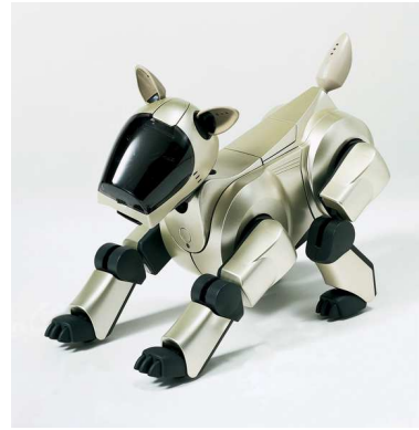
Figure 1.9: Robotic systems. (a) Spirit, one of the two Mars Exploratory Rovers that landed on Mars in January 2004. (b) The Sony AIBO Entertainment Robot, one of the first entertainment robots to be mass-marketed. Both robots make use of feedback between sensors, actuators and computation to function in unknown environments. (Photographs courtesy of Jet Propulsion Laboratory and Sony Electronics, Inc.)
