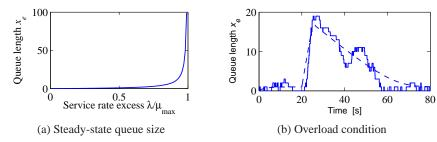
**Figure 2.19:** Queuing dynamics. (a) The steady-state queue length as a function of  $\lambda/\mu_{max}$ . (b) The behavior of the queue length when there is a temporary overload in the system. The solid line shows a realization of an event-based simulation, and the dashed line shows the behavior of the flow model (2.29).
