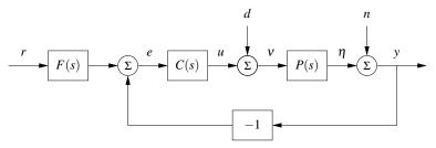
**Figure 8.7:** Block diagram of a feedback system. The inputs to the system are the reference signal r, the process disturbance d and the measurement noise n. The remaining signals in the system can all be chosen as possible outputs, and transfer functions can be used to relate the system inputs to the other labeled signals.
