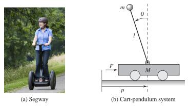
**Figure 6.2:** Balance system. The Segway Personal Transporter shown in (a) is an example of a balance system that uses torque applied to the wheels to keep the rider upright. A simplified diagram for a balance system is shown in (b). The system consists of a mass m on a rod of length l connected by a pivot to a cart with mass M.
