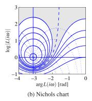
**Figure 12.16:** Hall and Nichols charts. The Hall chart is a Nyquist plot with curves for constant gain and phase of the complementary sensitivity function T. The Nichols chart is the conformal map of the Hall chart under the transformation  $N = \log L$  (with the scale flipped). The dashed curve is the line where  $|T(i\omega)| = 1$ , and the shaded region corresponding to loop transfer functions whose complementary sensitivity changes by no more than  $\pm 10\%$  is shaded.
