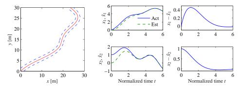
**Figure 7.6:** Simulation of an observer for a vehicle driving on a curvy road (left). The observer has an initial velocity error. The plots on the middle show the lateral deviation  $x_1$ , the lateral velocity  $x_2$  by solid lines and their estimates  $\hat{x}_1$  and  $\hat{x}_2$  by dashed lines. The plots on the right show the estimation errors.
