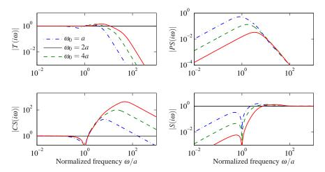
**Figure 12.15:** Nanopositioner control using active damping. Gain curves for the Gang of Four for PID control of the nanopositioner designed for  $\omega_0 = a$  (dash-dotted), 2a (dashed), and 4a (solid). The controller has high-frequency roll-off and has been designed to give active damping of the oscillatory mode. The different curves correspond to different choices of magnitudes of the poles, parameterized by  $\omega_0$  in equation (12.19).
