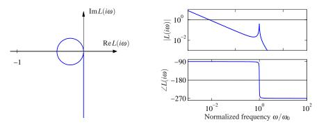
**Figure 9.12:** Nyquist and Bode plots of the loop transfer function for the AFM system (9.7) with an integral controller. The frequency in the Bode plot is normalized by a. The parameters are  $\zeta = 0.01$  and  $k_i = 0.008$ .
