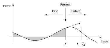
**Figure 1.17:** Action of a PID controller. At time t, the proportional term depends on the instantaneous value of the error. The integral portion of the feedback is based on the integral of the error up to time t (shaded portion). The derivative term provides an estimate of the growth or decay of the error over time by looking at the rate of change of the error.  $T_d$  represents the approximate amount of time in which the error is projected forward (see text).
