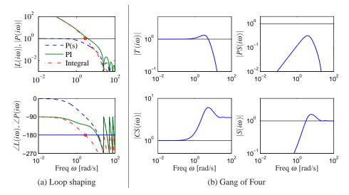
**Figure 11.10:** Loop-shaping design of a controller for an atomic force microscope in tapping mode. (a) Bode plots of the process (dashed), the loop transfer function for an integral controller with critical gain (dotted) and a PI controller (solid) adjusted to give reasonable robustness. (b) Gain curves for the Gang of Four for the system.
