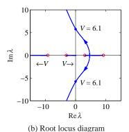
**Figure 4.18:** Stability plots for a bicycle moving at constant velocity. The plot in (a) shows the real part of the system eigenvalues as a function of the bicycle velocity v. The system is stable when all eigenvalues have negative real part (shaded region). The plot in (b) shows the locus of eigenvalues on the complex plane as the velocity v is varied and gives a different view of the stability of the system. This type of plot is called a *root locus diagram*.
