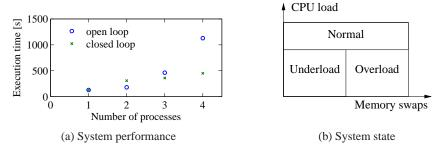
**Figure 2.20:** Illustration of feedback in the virtual memory system of the IBM/370. (a) The effect of feedback on execution times in a simulation, following [BG68]. Results with no feedback are shown with  $\circ$ , and results with feedback with x. Notice the dramatic decrease in execution time for the system with feedback. (b) How the three states are obtained based on process measurements.
