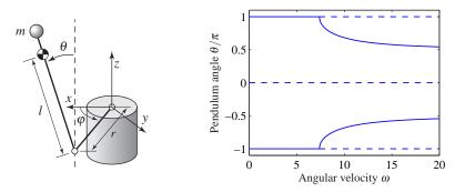
Consider the situation when the pendulum arm is spinning with constant rate. The system has multiple equilibrium points that depend on the angular velocity  $\omega$ , as shown in the bifurcation diagram on the right.
