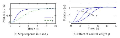
**Figure 6.12:** Step response for a vectored thrust aircraft. The plot in (a) shows the x and y positions of the aircraft when it is commanded to move 1 m in each direction. In (b) the x motion is shown for control weights  $\rho = 1$ ,  $10^2$ ,  $10^4$ . A higher weight of the input term in the cost function causes a more sluggish response.
