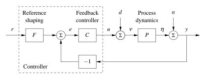
**Figure 8.1:** A block diagram for a feedback control system. The reference signal r is fed through a reference shaping block, which produces the signal that will be tracked. The error between this signal and the output is fed to a controller, which produces the input to the process. Disturbances and noise are included as external signals at the input and output of the process dynamics.
