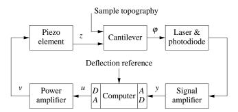
**Figure 3.15:** Block diagram of the system for vertical positioning of the cantilever for an atomic force microscope in contact mode. The control system attempts to keep the cantilever deflection equal to its reference value. Cantilever deflection is measured, amplified and converted to a digital signal, then compared with its reference value. A correcting signal is generated by the computer, converted to analog form, amplified and sent to the piezo element.
