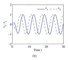
**Figure 4.5:** Phase portrait and time domain simulation for a system with a limit cycle. The phase portrait (a) shows the states of the solution plotted for different initial conditions. The limit cycle corresponds to a closed loop trajectory. The simulation (b) shows a single solution plotted as a function of time, with the limit cycle corresponding to a steady oscillation of fixed amplitude.
