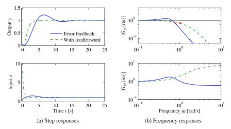
**Figure 11.5:** Reference signal responses. The responses in process output y and control signal u to a unit step in the reference signal r are shown in (a), and the gain curves of  $G_{yr}$  and  $G_{ur}$  are shown in (b). Results with PI control with error feedback are shown by solid lines, and the dashed lines show results for a controller with a feedforward compensator.
