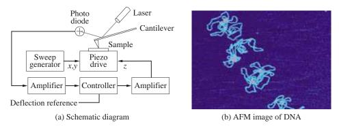
**Figure 3.14:** Atomic force microscope. (a) A schematic diagram of an atomic force microscope, consisting of a piezo drive that scans the sample under the AFM tip. A laser reflects off of the cantilever and is used to measure the detection of the tip through a feedback controller. (b) An AFM image of strands of DNA. (Image courtesy Veeco Instruments.)
