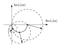
**Figure 12.6:** Robustness for a cruise controller. On the left the maximum relative error 1/|T| (solid) and the absolute error |P|/|T| (dashed) for the process uncertainty  $\Delta$ . The Nyquist curve is shown on the right as a solid line. The dashed circles show permissible perturbations in the process dynamics,  $|\Delta| = |P|/|T|$ , at the frequencies  $\omega = 0$ , 0.0142 and 0.05.
