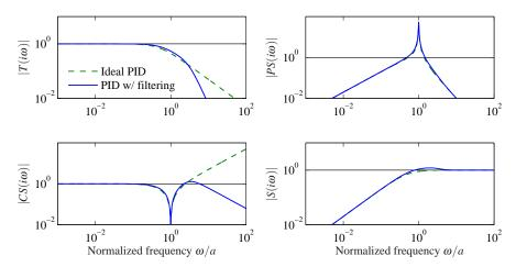
**Figure 12.14:** Nanopositioning system control via cancellation of the fast process pole. Gain plots for the Gang of Four for PID control with second-order filtering (12.17) are shown by solid lines, and the dashed lines show results for an ideal PID controller without filtering (12.16).
