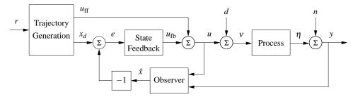
**Figure 7.10:** Block diagram of a controller based on a structure with two degrees of freedom which combines feedback and feedforward. The controller consists of a trajectory generator, state feedback and an observer. The trajectory generation subsystem computes a feedforward command  $u_{\rm ff}$  along with the desired state  $x_d$ . The state feedback controller uses the estimated state and desired state to compute a corrective input  $u_{\rm fb}$ .
