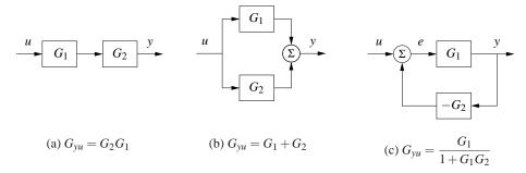
**Figure 8.6:** Interconnections of linear systems. Series (a), parallel (b) and feedback (c) connections are shown. The transfer functions for the composite systems can be derived by algebraic manipulations assuming exponential functions for all signals.
