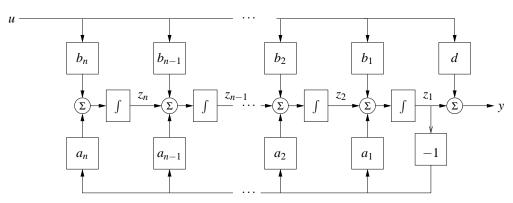
**Figure 7.3:** Block diagram of a system in observable canonical form. The states of the system are represented by individual integrators whose inputs are a weighted combination of the next integrator in the chain, the first state (rightmost integrator) and the system input. The output is a combination of the first state and the input.
