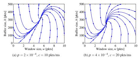
**Figure 4.10:** Phase portraits for a congestion control protocol running with N = 60 identical source computers. The equilibrium values correspond to a fixed window at the source, which results in a steady-state buffer size and corresponding transmission rate. A faster link (b) uses a smaller buffer size since it can handle packets at a higher rate.
