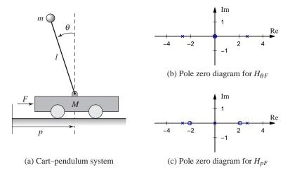
**Figure 8.5:** Poles and zeros for a balance system. The balance system (a) can be modeled around its vertical equilibrium point by a fourth order linear system. The poles and zeros for the transfer functions  $H_{\theta F}$  and  $H_{pF}$  are shown in (b) and (c), respectively.
