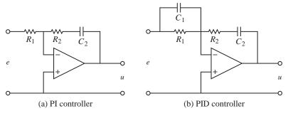
**Figure 10.13:** Schematic diagrams for PI and PID controllers using op amps. The circuit in (a) uses a capacitor in the feedback path to store the integral of the error. The circuit in (b) adds a filter on the input to provide derivative action.
