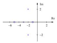
**Figure 8.4:** A pole zero diagram for a transfer function with zeros at -5 and -1 and poles at -3 and  $-2 \pm 2j$ . The circles represent the locations of the zeros, and the crosses the locations of the poles. A complete characterization requires we also specify the gain of the system.
