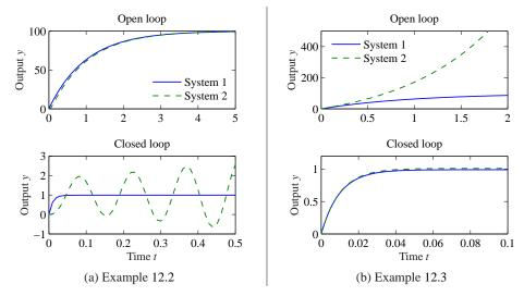
**Figure 12.3:** Determining when two systems are close. The plots in (a) show a situation when the open loop responses are almost identical, but the closed loop responses are very different. The processes are given by equation (12.1) with k = 100 and T = 0.025. The plots in (b) show the opposite situation: the systems are different in open loop but similar in closed loop. The processes are given by equation (12.2) with k = 100.
