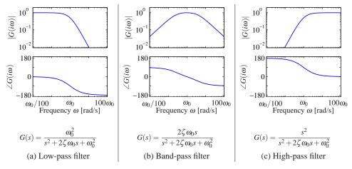
**Figure 8.15:** Bode plots for low-pass, band-pass and high-pass filters. The top plots are the gain curves and the bottom plots are the phase curves. Each system passes frequencies in a different range and attenuates frequencies outside of that range.
