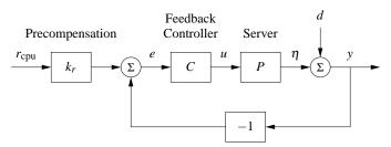
**Figure 6.13:** Feedback control of a web server. The controller sets the values of the web server parameters based on the difference between the nominal parameters (determined by  $k_r r$ ) and the current load  $y_{\text{cpu}}$ . The disturbance d represents the load due to other processes running on the server. Note that the measurement is taken after the disturbance so that we measure the total load on the server.
