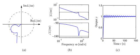
**Figure 9.11:** System with good gain and phase margins but a poor stability margin. Nyquist (a) and Bode (b) plots of the loop transfer function and step response (c) for a system with good gain and phase margins but with a poor stability margin. The Nyquist plot shows on the portion of the curve corresponding to  $\omega > 0$ .
