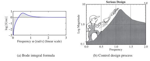
**Figure 11.14:** Interpretation of the *waterbed effect*. The function  $\log |S(i\omega)|$  is plotted versus  $\omega$  in linear scales in (a). According to Bode's integral formula (11.19), the area of  $\log |S(i\omega)|$  above zero must be equal to the area below zero. Gunter Stein's interpretation of design as a trade-off of sensitivities at different frequencies is shown in (b) (from [Ste03]).
