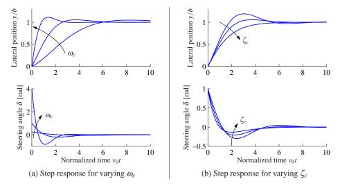
**Figure 6.6:** State feedback control of a steering system. Step responses obtained with controllers designed with  $\zeta_c = 0.7$  and  $\omega_c = 0.5$ , 1 and 2 [rad/s] are shown in (a). Notice that response speed increases with increasing  $\omega_c$ , but that large  $\omega_c$  also give large initial control actions. Step responses obtained with a controller designed with  $\omega_c = 1$  and  $\zeta_c = 0.5$ , 0.7 and 1 are shown in (b).
