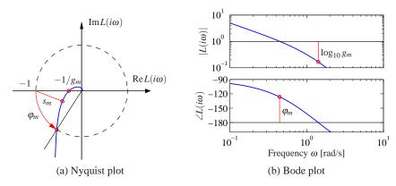
Figure 9.9: Stability margins. The gain margin  $g_m$  and phase margin  $\phi_m$  are shown on the the Nyquist plot (a) and the Bode plot (b). The gain margin corresponds to the smallest increase in gain that creates an encirclement, and the phase margin is the smallest change in phase that creates an encirclement. The Nyquist plot also shows the stability margin  $s_m$ , which is the shortest distance to the critical point -1.
