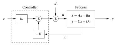
**Figure 6.5:** A feedback control system with state feedback. The controller uses the system state x and the reference input r to command the process through its input u. We model disturbances via the additive input d.
