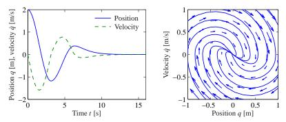
**Figure 2.2:** Illustration of a state model. A state model gives the rate of change of the state as a function of the state. The plot on the left shows the evolution of the state as a function of time. The plot on the right shows the evolution of the states relative to each other, with the velocity of the state denoted by arrows.
