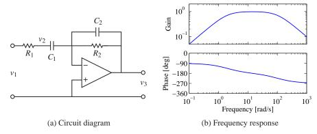
**Figure 5.12:** Active band-pass filter. The circuit diagram (a) shows an op amp with two *RC* filters arranged to provide a band-pass filter. The plot in (b) shows the gain and phase of the filter as a function of frequency. Note that the phase starts at -90° due to the negative gain of the operational amplifier.
