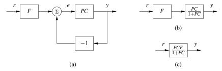
**Figure 8.8:** Example of block diagram algebra. The results from multiplying the process and controller transfer functions (from Figure 8.7) are shown in (a). Replacing the feedback loop with its transfer function equivalent yields (b), and finally multiplying the two remaining blocks gives the reference to output representation in (c).
