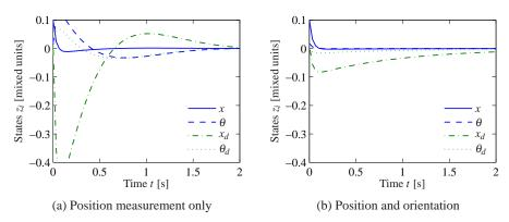
**Figure 7.9:** Kalman filter design for a vectored thrust aircraft. In the first design (a) only the lateral position of the aircraft is measured. Adding a direct measurement of the roll angle produces a much better observer (b). The initial condition for both simulations is (0.1, 0.0175, 0.01, 0).
