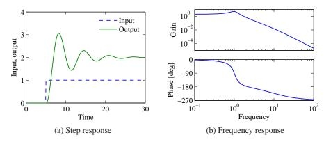
**Figure 2.4:** Input/output response of a linear system. The step response (a) shows the output of the system due to an input that changes from 0 to 1 at time t = 5 s. The frequency response (b) shows the amplitude gain and phase change due to a sinusoidal input at different frequencies.
