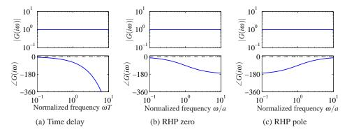
**Figure 9.13:** Bode plots of systems that are not minimum phase. (a) Time delay  $G(s) = e^{-sT}$ , (b) system with a right half-plane (RHP) zero G(s) = (a-s)/(a+s) and (c) system with right half-plane pole. The corresponding minimum phase system has the transfer function G(s) = 1 in all cases, the phase curves for that system are shown as dashed lines.
