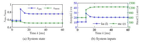
**Figure 6.14:** Web server with LQR control. The plot in (a) shows the state of the system under a change in external load applied at k = 10 ms. The corresponding web server parameters (system inputs) are shown in (b). The controller is able to reduce the effect of the disturbance by approximately 40%.
