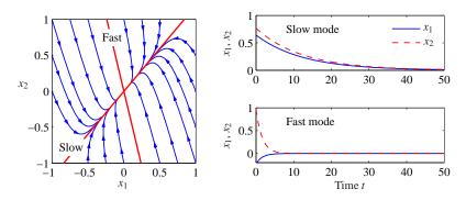
**Figure 5.5:** The notion of modes for a second-order system with real eigenvalues. The left figure shows the phase portrait and the modes corresponding to solutions that start on the eigenvectors (bold lines). The corresponding time functions are shown on the right.
