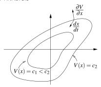
**Figure 4.13:** Geometric illustration of Lyapunov's stability theorem. The closed contours represent the level sets of the Lyapunov function V(x) = c. If dx/dt points inward to these sets at all points along the contour, then the trajectories of the system will always cause V(x) to decrease along the trajectory.
