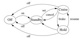
**Figure 3.4:** Finite state machine for cruise control system. The figure on the left shows some typical buttons used to control the system. The controller can be in one of four modes, corresponding to the nodes in the diagram on the right. Transition between the modes is controlled by pressing one of the five buttons on the cruise control interface: on, off, set, resume or cancel.
