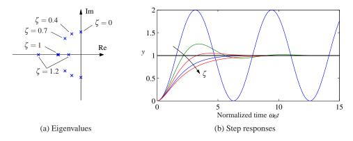
**Figure 6.8:** Step response for a second-order system. Normalized step responses h for the system (6.23) for  $\zeta = 0$ , 0.4, 0.7, 1 and 1.2. As the damping ratio is increased, the rise time of the system gets longer, but there is less overshoot. The horizontal axis is in scaled units  $\omega_0 t$ ; higher values of  $\omega_0$  result in a faster response (rise time and settling time).
