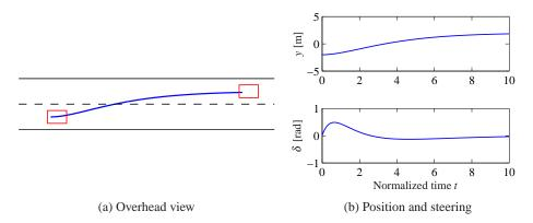
**Figure 11.4:** Feedforward control for vehicle steering. The plot on the left shows the trajectory generated by the controller for changing lanes. The plots on the right show the lateral deviation y (top) and the steering angle  $\delta$  (bottom) for a smooth lane change control using feedforward (based on the linearized model).
