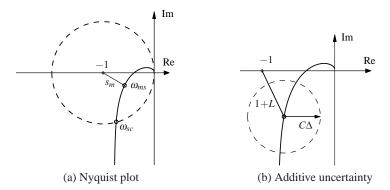
**Figure 12.5:** Robust stability using the Nyquist criterion. (a) This plot shows that the shortest distance to the critical point  $s_m$  is a robustness measure. (b) This plot shows the Nyquist curve of a nominal loop transfer function and its uncertainty caused by additive process variations  $\Delta$ .
