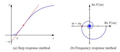
**Figure 10.7:** Ziegler–Nichols step and frequency response experiments. The unit step response in (a) is characterized by the parameters a and  $\tau$ . The frequency response method (b) characterizes process dynamics by the point where the Nyquist curve of the process transfer function first intersects the negative real axis and the frequency  $\omega_c$  where this occurs.
