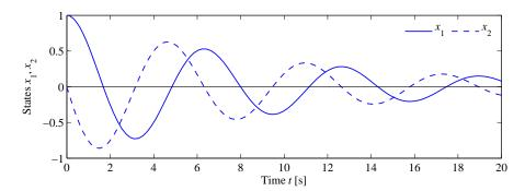
**Figure 4.1:** Response of the damped oscillator to the initial condition  $x_0 = (1,0)$ . The solution is unique for the given initial conditions and consists of an oscillatory solution for each state, with an exponentially decaying magnitude.
