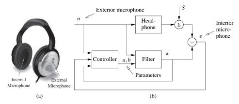
**Figure 4.19:** Headphones with noise cancellation. Noise is sensed by the exterior microphone (a) and sent to a filter in such a way that it cancels the noise that penetrates the head phone (b). The filter parameters a and b are adjusted by the controller. S represents the input signal to the headphones.
