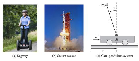
**Figure 2.5:** Balance systems. (a) Segway Personal Transporter, (b) Saturn rocket and (c) inverted pendulum on a cart. Each of these examples uses forces at the bottom of the system to keep it upright.
