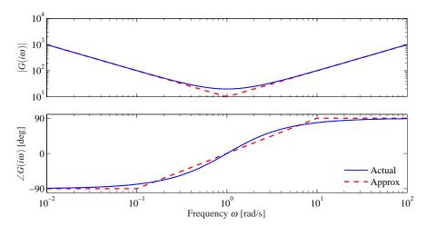
**Figure 8.11:** Bode plot of the transfer function C(s) = 20 + 10/s + 10s corresponding to an ideal PID controller. The top plot is the gain curve and the bottom plot is the phase curve. The dashed lines show straight-line approximations of the gain curve and the corresponding phase curve.
