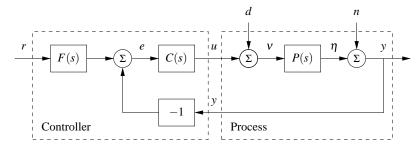
**Figure 12.9:** Block diagram of a basic feedback loop. The external signals are the reference signal r, the load disturbance d and the measurement noise n. The process output is y, and the control signal is u. The process P may include unmodeled dynamics, such as additive perturbations.
