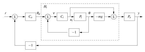
**Figure 11.17:** Inner/outer control design for a vectored thrust aircraft. The inner loop  $H_i$  controls the roll angle of the aircraft using the vectored thrust. The outer loop controller  $C_o$  commands the roll angle to regulate the lateral position. The process dynamics are decomposed into inner loop  $(P_i)$  and outer loop  $(P_o)$  dynamics, which combine to form the full dynamics for the aircraft.
