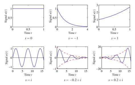
**Figure 8.2:** Examples of exponential signals. The top row corresponds to exponential signals with a real exponent, and the bottom row corresponds to those with complex exponents. The dashed line in the last two cases denotes the bounding envelope for the oscillatory signals. In each case, if the real part of the exponent is negative then the signal decays, while if the real part is positive then it grows.
