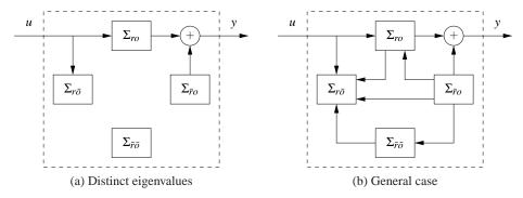
**Figure 7.12:** Kalman's decomposition of a linear system. The decomposition in (a) is for a system with distinct eigenvalues and the one in (b) is the general case. The system is broken into four subsystems, representing the various combinations of reachable and observable states. The input/output relationship only depends on the subset of states that are both reachable and observable.
