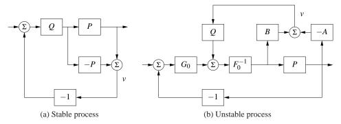
**Figure 12.8:** Youla parameterization. Block diagrams of Youla parameterizations for a stable system (a) and an unstable system (b). Notice that the signal  $\nu$  is zero in steady state.
