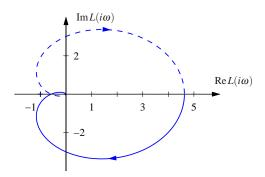
**Figure 9.4:** Nyquist plot for a third-order transfer function. The Nyquist plot consists of a trace of the loop transfer function  $L(s) = 1/(s+a)^3$ . The solid line represents the portion of the transfer function along the positive imaginary axis, and the dashed line the negative imaginary axis. The outer arc of the D contour maps to the origin.
