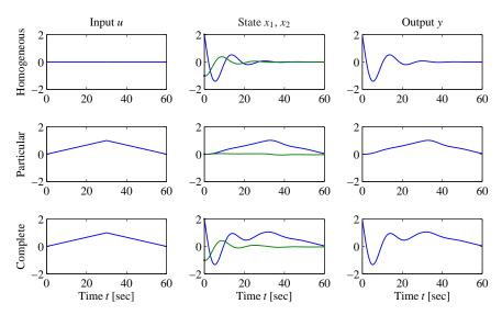
**Figure 5.1:** Superposition of homogeneous and particular solutions. The first row shows the input, state and output corresponding to the initial condition response. The second row shows the same variables corresponding to zero initial condition but nonzero input. The third row is the complete solution, which is the sum of the two individual solutions.
