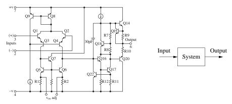
**Figure 2.3:** Illustration of the input/output view of a dynamical system. The figure on the left shows a detailed circuit diagram for an electronic amplifier; the one on the right is its representation as a block diagram.
