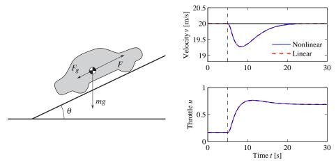
**Figure 5.14:** Simulated response of a vehicle with PI cruise control as it climbs a hill with a slope of  $4^{\circ}$ . The solid line is the simulation based on a nonlinear model, and the dashed line shows the corresponding simulation using a linear model. The controller gains are  $k_p = 0.5$  and  $k_i = 0.1$ .
