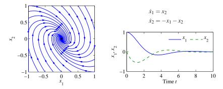
**Figure 4.8:** Phase portrait and time domain simulation for a system with a single asymptotically stable equilibrium point. The equilibrium point  $x_e$  at the origin is asymptotically stable since the trajectories converge to this point as  $t \to \infty$ .
