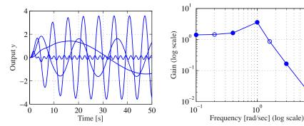
**Figure 2.10:** A frequency response (gain only) computed by measuring the response of individual sinusoids. The figure on the left shows the response of the system as a function of time to a number of different unit magnitude inputs (at different frequencies). The figure on the right shows this same data in a different way, with the magnitude of the response plotted as a function of the input frequency. The filled circles correspond to the particular frequencies shown in the time responses.
