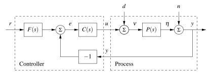
**Figure 11.1:** Block diagram of a basic feedback loop with two degrees of freedom. The controller has a feedback block C and a feedforward block F. The external signals are the reference signal r, the load disturbance d and the measurement noise n. The process output is  $\eta$ , and the control signal is u.
