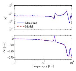
**Figure 8.17:** Frequency response of a preloaded piezoelectric drive for an atomic force microscope. The Bode plot shows the response of the measured transfer function (solid) and the fitted transfer function (dashed).
