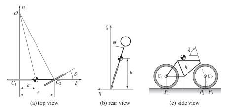
**Figure 3.5:** Schematic views of a bicycle. The steering angle is  $\delta$ , and the roll angle is  $\varphi$ . The center of mass has height h and distance a from a vertical through the contact point  $P_1$  of the rear wheel. The wheel base is b, and the trail is c.
