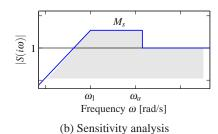
**Figure 11.15:** X-29 flight control system. The aircraft makes use of forward swept wings and a set of canards on the fuselage to achieve high maneuverability (a). The desired sensitivity for the closed loop system is shown in (b). We seek to use our control authority to shape the sensitivity curve so that we have low sensitivity (good performance) up to frequency  $\omega_1$  by creating higher sensitivity up to our actuator bandwidth  $\omega_a$ .
