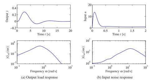
**Figure 11.7:** Disturbance responses. The time and frequency responses of process output y to load disturbance d are shown in (a) and the responses of control signal u to measurement noise n are shown in (b).
