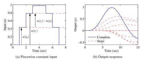
**Figure 5.2:** Response to piecewise constant inputs. A piecewise constant signal can be represented as a sum of step signals (a), and the resulting output is the sum of the individual outputs (b).
