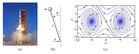
**Figure 4.4:** Equilibrium points for an inverted pendulum. An inverted pendulum is a model for a class of balance systems in which we wish to keep a system upright, such as a rocket (a). Using a simplified model of an inverted pendulum (b), we can develop a phase portrait that shows the dynamics of the system (c). The system has multiple equilibrium points, marked by the solid dots along the  $x_2 = 0$  line.
