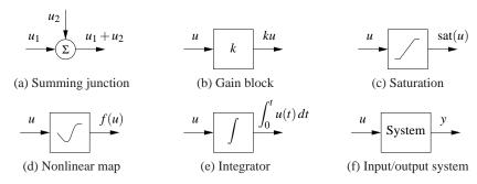
**Figure 2.12:** Standard block diagram elements. The arrows indicate the inputs and outputs of each element, with the mathematical operation corresponding to the blocked labeled at the output. The system block (f) represents the full input/output response of a dynamical system.
