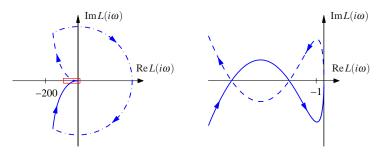
**Figure 9.7:** Nyquist curve for the loop transfer function  $L(s) = \frac{3(s+1)^2}{s(s+6)^2}$ . The plot on the right is an enlargement of the box around the origin of the plot on the left. The Nyquist curve intersects the negative real axis twice but has no net encirclements of -1.
