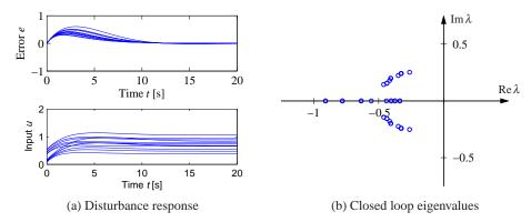
**Figure 12.1:** Responses of the cruise control system to a slope increase of 3° (a) and the eigenvalues of the closed loop system (b). Model parameters are swept over a wide range.
