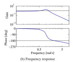
**Figure 5.11:** Response of a linear system to a sinusoid. (a) A sinusoidal input of magnitude  $A_u$  (dashed) gives a sinusoidal output of magnitude  $A_y$  (solid), delayed by  $\Delta T$  seconds. (b) Frequency response, showing gain and phase. The gain is given by the ratio of the output amplitude to the input amplitude,  $M = A_y/A_u$ . The phase lag is given by  $\theta = -2\pi\Delta T/T$ ; it is negative for the case shown because the output lags the input.
