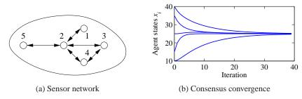
**Figure 2.21:** Consensus protocols for sensor networks. (a) A simple sensor network with five nodes. In this network, node 1 communicates with node 2 and node 2 communicates with nodes 1, 3, 4, 5, etc. (b) A simulation demonstrating the convergence of the consensus protocol (2.31) to the average value of the initial conditions.
