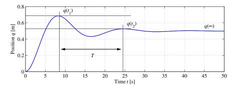
**Figure 2.14:** Step response for a spring-mass system. The magnitude of the step input is  $F_0 = 20$  N. The period of oscillation T is determined by looking at the time between two subsequent local maxima in the response. The period combined with the steady-state value  $q(\infty)$  and the relative decrease between local maxima can be used to estimate the parameters in a model of the system.
