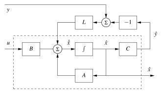
**Figure 7.5:** Block diagram of the observer. The observer takes the signals y and u as inputs and produces an estimate x. Notice that the observer contains a copy of the process model that is driven by  $y - \hat{y}$  through the observer gain L.
