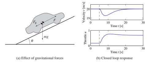
**Figure 3.3:** Car with cruise control encountering a sloping road. A schematic diagram is shown in (a), and (b) shows the response in speed and throttle when a slope of  $4^{\circ}$  is encountered. The hill is modeled as a net change of  $4^{\circ}$  in hill angle  $\theta$ , with a linear change in the angle between t = 5 and t = 6. The PI controller has proportional gain is  $k_p = 0.5$ , and the integral gain is  $k_i = 0.1$ .
