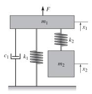
The disturbing vibration is a sinusoidal force acting on mass  $m_1$ , and the damper consists of the mass  $m_2$  and the spring  $k_2$ . Show that the transfer function from disturbance force to height  $x_1$  of the mass  $m_1$  is
