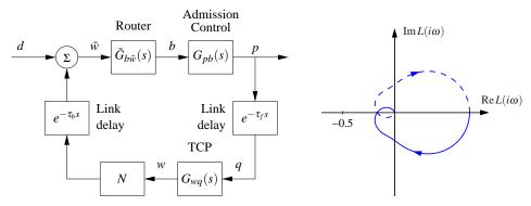
Figure 9.6: Internet congestion control. A set of N sources using TCP/Reno send messages through a single router with admission control (left). Link delays are included for the forward and backward directions. The Nyquist plot for the loop transfer function is shown on the right.
