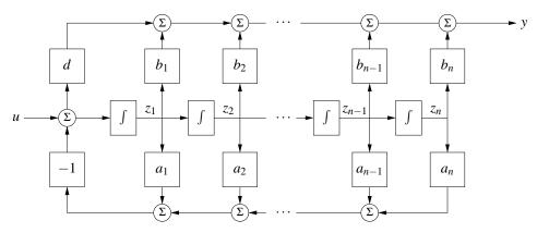
**Figure 6.4:** Block diagram for a system in reachable canonical form. The individual states of the system are represented by a chain of integrators whose input depends on the weighted values of the states. The output is given by an appropriate combination of the system input and other states.
