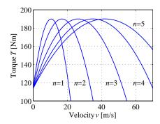
**Figure 3.2:** Torque curves for typical car engine. The graph on the left shows the torque generated by the engine as a function of the angular velocity of the engine, while the curve on the right shows torque as a function of car speed for different gears.
