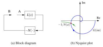
**Figure 9.16:** Describing function analysis. A feedback connection between a static nonlinearity and a linear system is shown in (a). The linear system is characterized by its transfer function L(s), which depends on frequency, and the nonlinearity by its describing function N(a), which depends on the amplitude a of its input. The Nyquist plot of  $L(i\omega)$  and the plot of the -1/N(a) are shown in (b). The intersection of the curves represents a possible limit cycle.
