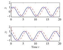
**Figure 4.12:** Solution curves for a stable limit cycle. The phase portrait on the left shows that the trajectory for the system rapidly converges to the stable limit cycle. The starting points for the trajectories are marked by circles in the phase portrait. The time domain plots on the right show that the states do not converge to the solution but instead maintain a constant phase error.
