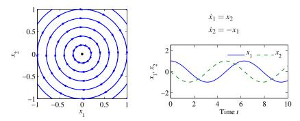
**Figure 4.7:** Phase portrait and time domain simulation for a system with a single stable equilibrium point. The equilibrium point  $x_e$  at the origin is stable since all trajectories that start near  $x_e$  stay near  $x_e$ .
