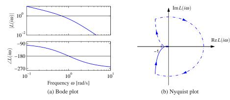
**Figure 9.5:** Sketching Nyquist and Bode plots. The loop transfer function is  $L(s) = 1/(s(s+1)^2)$ . The large semicircle is the map of the small semicircle of the  $\Gamma$  contour around the pole at the origin. The closed loop is stable because the Nyquist curve does not encircle the critical point. The point where the phase is  $-180^{\circ}$  is marked with a circle in the Bode plot.
