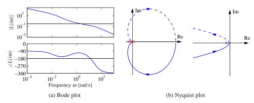
**Figure 11.19:** Inner/outer loop controller for a vectored thrust aircraft. The Bode plot (a) and Nyquist plot (b) for the transfer function for the combined inner and outer loop transfer functions are shown. The system has a phase margin of 68° and a gain margin of 6.2.
