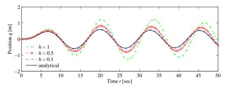
**Figure 2.9:** Simulation of the forced spring—mass system with different simulation time constants. The solid line represents the analytical solution. The dashed lines represent the approximate solution via the method of Euler integration, using decreasing step sizes.
