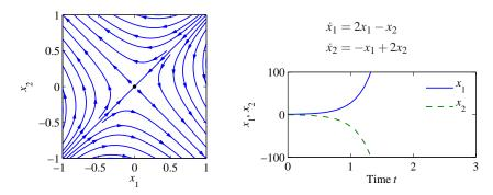
**Figure 4.9:** Phase portrait and time domain simulation for a system with a single unstable equilibrium point. The equilibrium point  $x_e$  at the origin is unstable since not all trajectories that start near  $x_e$  stay near  $x_e$ . The sample trajectory on the right shows that the trajectories very quickly depart from zero.
