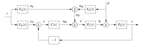
**Figure 11.3:** Block diagram of a system with feedforward compensation for improved response to reference signals and measured disturbances (2 DOF system). Three feedforward elements are present:  $F_m(s)$  sets the desired output value,  $F_u(s)$  generates the feedforward command  $u_{\rm fr}$  and  $F_d(s)$  attempts to cancel disturbances.
