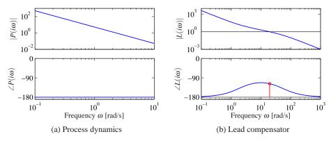
**Figure 11.12:** Control design for a vectored thrust aircraft using lead compensation. The Bode plot for the open loop process P is shown in (a) and the loop transfer function L = PC using a lead compensator in (b). Note the phase lead in the crossover region near  $\omega = 100 \text{ rad/s}$ .
