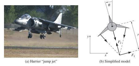
**Figure 2.17:** Vectored thrust aircraft. The Harrier AV-8B military aircraft (a) redirects its engine thrust downward so that it can "hover" above the ground. Some air from the engine is diverted to the wing tips to be used for maneuvering. As shown in (b), the net thrust on the aircraft can be decomposed into a horizontal force  $F_1$  and a vertical force  $F_2$  acting at a distance r from the center of mass.
