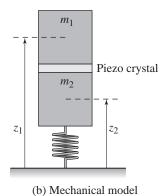
**Figure 3.16:** Modeling of an atomic force microscope. (a) A measured step response. The top curve shows the voltage u applied to the drive amplifier (50 mV/div), the middle curve is the output  $V_p$  of the power amplifier (500 mV/div) and the bottom curve is the output y of the signal amplifier (500 mV/div). The time scale is 25  $\mu$ s/div. Data have been supplied by Georg Schitter. (b) A simple mechanical model for the vertical positioner and the piezo crystal.
