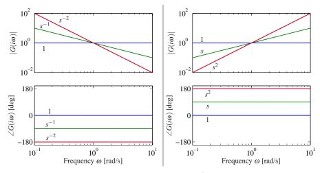
**Figure 8.12:** Bode plots of the transfer functions  $G(s) = s^k$  for k = -2, -1, 0, 1, 2. On a loglog scale, the gain curve is a straight line with slope k. Using a log-linear scale, the phase curves for the transfer functions are constants, with phase equal to  $90^\circ \times k$
