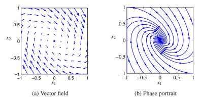
**Figure 4.3:** Phase portraits. (a) This plot shows the vector field for a planar dynamical system. Each arrow shows the velocity at that point in the state space. (b) This plot includes the solutions (sometimes called streamlines) from different initial conditions, with the vector field superimposed.
