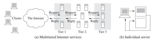
**Figure 1.10:** A multitier system for services on the Internet. In the complete system shown schematically in (a), users request information from a set of computers (tier 1), which in turn collect information from other computers (tiers 2 and 3). The individual server shown in (b) has a set of reference parameters set by a (human) system operator, with feedback used to maintain the operation of the system in the presence of uncertainty. (Based on Hellerstein et al. [HDPT04].)
