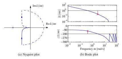
**Figure 10.5:** Integral control for AFM in tapping mode. An integral controller is designed based on the slope of the process transfer function at 0. The controller gives good robustness properties based on a very simple analysis.
