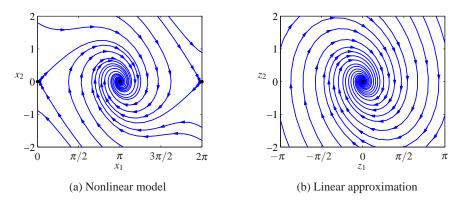
**Figure 4.11:** Comparison between the phase portraits for the full nonlinear systems (a) and its linear approximation around the origin (b). Notice that near the equilibrium point at the center of the plots, the phase portraits (and hence the dynamics) are almost identical.
