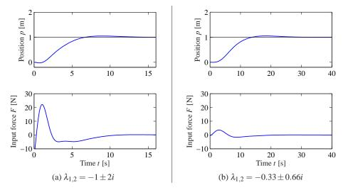
**Figure 6.11:** State feedback control of a balance system. The step response of a controller designed to give fast performance is shown in (a). Although the response characteristics (top left) look very good, the input magnitude (bottom left) is very large. A less aggressive controller is shown in (b). Here the response time is slowed down, but the input magnitude is much more reasonable. Both step responses are applied to the linearized dynamics.
