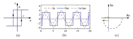
**Figure 9.17:** Describing function analysis for a relay with hysteresis. The input/output relation of the hysteresis is shown in (a) and the input with amplitude a = 2, the output and its first harmonic are shown in (b). The Nyquist plots of the transfer function  $L(s) = (s+1)^{-4}$  and the negative of the inverse describing function for the relay with b = 3 and c = 1 are shown in (c).
