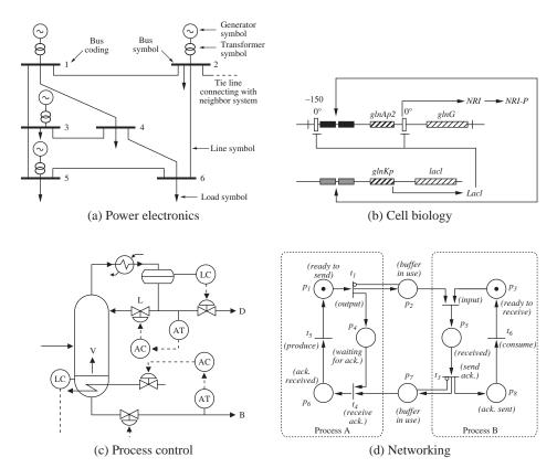
**Figure 2.11:** Schematic diagrams for different disciplines. Each diagram is used to illustrate the dynamics of a feedback system: (a) electrical schematics for a power system [Kun93], (b) a biological circuit diagram for a synthetic clock circuit [ASMN03], (c) a process diagram for a distillation column [SEM04] and (d) a Petri net description of a communication protocol.
