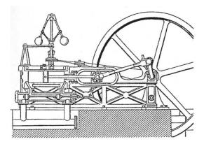
**Figure 1.2:** The centrifugal governor and the steam engine. The centrifugal governor on the left consists of a set of flyballs that spread apart as the speed of the engine increases. The steam engine on the right uses a centrifugal governor (above and to the left of the flywheel) to regulate its speed. (Credit: Machine a Vapeur Horizontale de Philip Taylor [1828].)
