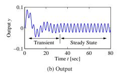
**Figure 5.8:** Transient versus steady-state response. The input to a linear system is shown in (a), and the corresponding output with x(0) = 0 is shown in (b). The output signal initially undergoes a transient before settling into its steady-state behavior.
