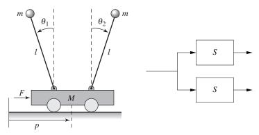
**Figure 6.3:** An unreachable system. The cart–pendulum system shown on the left has a single input that affects two pendula of equal length and mass. Since the forces affecting the two pendula are the same and their dynamics are identical, it is not possible to arbitrarily control the state of the system. The figure on the right is a block diagram representation of this situation.
