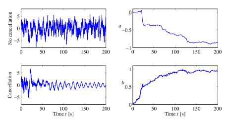
**Figure 4.20:** Simulation of noise cancellation. The top left figure shows the headphone signal without noise cancellation, and the bottom left figure shows the signal with noise cancellation. The right figures show the parameters *a* and *b* of the filter.
