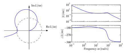
**Figure 12.11:** Observer-based control of steering. The Nyquist plot (left) and Bode plot (right) of the loop transfer function for vehicle steering with a controller based on state feedback and an observer. The controller provides stable operation, but with very low gain and phase margin.
