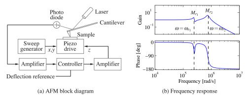
**Figure 5.13:** AFM frequency response. (a) A block diagram for the vertical dynamics of an atomic force microscope in contact mode. The plot in (b) shows the gain and phase for the piezo stack. The response contains two frequency peaks at resonances of the system, along with an antiresonance at  $\omega=268$  krad/s. The combination of a resonant peak followed by an antiresonance is common for systems with multiple lightly damped modes.
