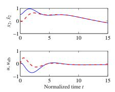
**Figure 7.8:** Simulation of a vehicle driving on a curvy road with a controller based on state feedback and an observer. The left plot shows the lane boundaries (dotted), the vehicle position (solid) and its estimate (dashed), the upper right plot shows the velocity (solid) and its estimate (dashed), and the lower right plot shows the control signal using state feedback (solid) and the control signal using the estimated state (dashed).
