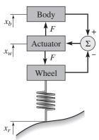
This model is called a *quarter car model*, and the car is approximated with two masses, one representing one fourth of the car body and the other a wheel. The
