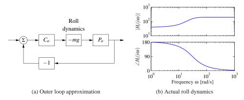
**Figure 11.18:** Outer loop control design for a vectored thrust aircraft. (a) The outer loop approximates the roll dynamics as a state gain -mg. (b) The Bode plot for the roll dynamics, indicating that this approximation is accurate up to approximately 10 rad/s.
