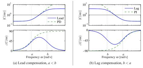
**Figure 11.9:** Frequency response for lead and lag compensators C(s) = k(s+a)/(s+b). Lead compensation (a) occurs when a < b and provides phase lead between  $\omega = a$  and  $\omega = b$ . Lag compensation (b) corresponds to a > b and provides low-frequency gain. PI control is a special case of lag compensation and PD control is a special case of lead compensation. PI/PD frequency responses are shown by dashed curves.
