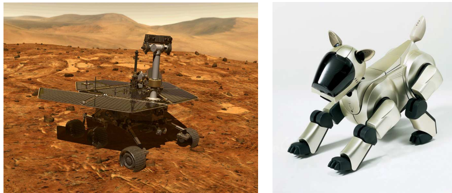
Figure 1.9: Robotic systems. (a) Spirit, one of the two Mars Exploratory Rovers that landed on Mars in January 2004. (b) The Sony AIBO Entertainment Robot, one of the first entertainment robots to be mass-marketed. Both robots make use of feedback between sensors, actuators and computation to function in unknown environments. (Photographs courtesy of Jet Propulsion Laboratory and Sony Electronics, Inc.)
