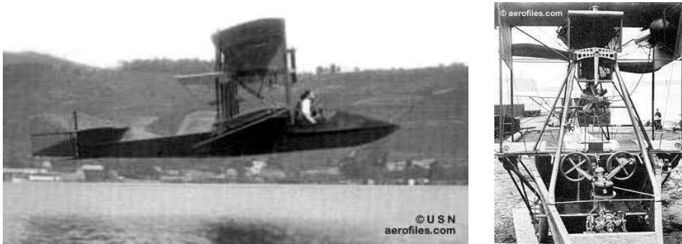
Figure 1.12: The Curtiss-Sperry E in 1912 (left) and a closeup of the Sperry Autopilot (right).
